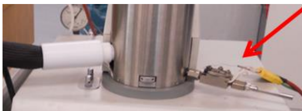
Figure 37: The heated exhaust of the furnace.
