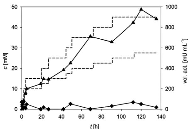
**Figure 5.** Controlled feeding of phloretin is useful to enhance the nothofagin concentration in the biocatalytic synthesis. *Reaction conditions:* 100 mU mL<sup>-1</sup> *OsCGT/GmSuSy*, 5 mM phloretin, 300 mM sucrose, 1 mM UDP. After acceptor substrate depletion, 5 mM phloretin and 50 mU mL<sup>-1</sup> *OsCGT/GmSuSy* were added. Symbols: phloretin added (black dashed), *OsCGT/GmSuSy* added (grey dashed), nothofagin (black), phloretin (grey)
