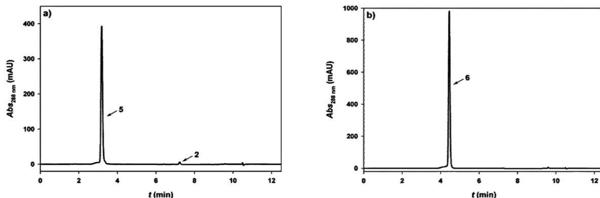
**Fig. S4** Reversed-phase C-18 HPLC-analysis of (a) davidioside (**5**) and (b) confusoside (**6**) after purification by preparative HPLC confirms them to be of high purity (>98% based on HPLC peak area).
