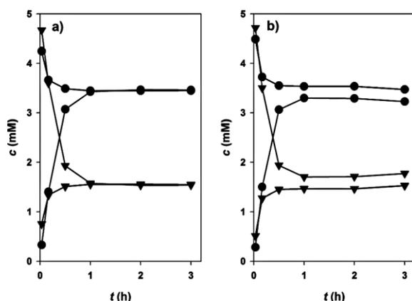
Fig. 2 Phlorizin (**3**) synthesis (grey, 5 mM **1** and **10**) and degradation (black, 5 mM **3** and **9**) by PcOGT (pH 6.5) level out at the same equilibrium concentrations. (a) **1** (triangles), **3** (circles); (b) **10** (triangles), **9** (circles).
