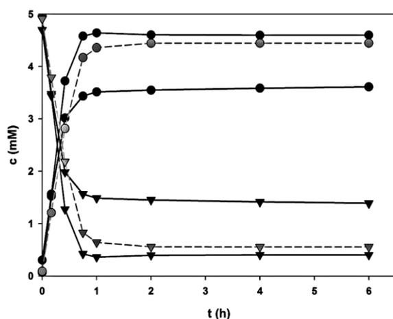
Fig. 4 *PcOGT* catalysed formation of **3** (circles) from 5 mM **1** (triangles) at pH 6.5: black: without *GmSuSy*, 5 mM **10**; dark grey: *GmSuSy*, 5 mM **10**; light grey (dashed): *GmSuSy*, 0.5 mM **9**.
