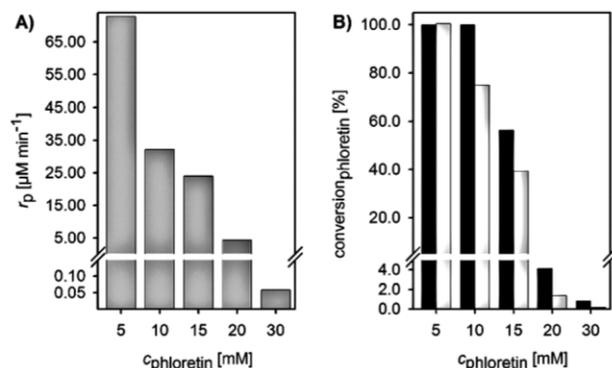
**Figure 4.** Batch conversions at different phloretin concentrations (100 mM sucrose, 0.5 mM UDP, 190 mU mL<sup>-1</sup> *OsCGT*, 120 mU mL<sup>-1</sup> *GmSuSy*); **A**) Nothofagin production rate decreases at elevated phloretin concentrations; **B**) final conversion of soluble (black) and total applied (grey) phloretin after 24 h is limited at high phloretin concentrations by substrate inhibition and solubility.
