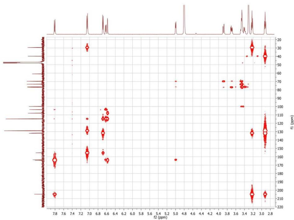
Fig. S15 2D HMBC-NMR of HPLC purified confusoside (6)
