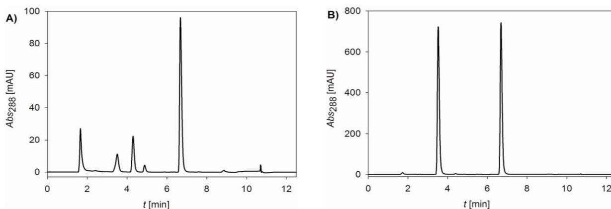
**Figure S2:** Separation of phloretin from its glycosides using RP-HPLC: A) mixture containing non-binding compounds like UDP(-glucose) (1.7 min), 3'-C-glycoside nothofagin (3.5 min), 2'-O-glycoside phlorizin (4.3 min), 4'-O-glycoside (4.9 min) and phloretin (6.7 min); B) partial phloretin conversion using *OsCGT* and *GmSuSy* contains only 3'-C-glycoside nothofagin (3.5 min), phloretin (6.7 min) and small amounts of UDP(-glucose)
