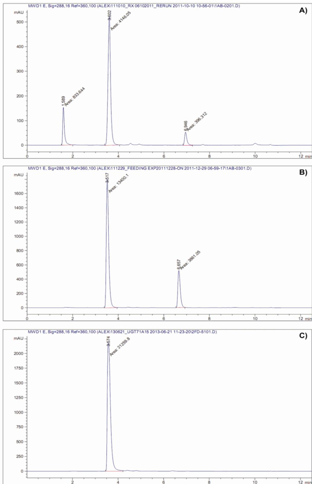
**Figure S8:** HPLC chromatograms (UV detection at 288 nm) showing nothofagin peak at ~3.5 min either from authentic standard A), after partial phloretin conversion in a coupled reaction of *OsCGT* and *GmSuSy* B) and after purification by reversed phase HPLC C).
