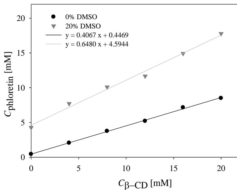
**Figure S3.** Phase solubility diagram of phloretin with increasing concentration of  $\beta$ -CD in HEPES buffer pH 7.5 at 30 °C in the absence and presence of 20% DMSO.
