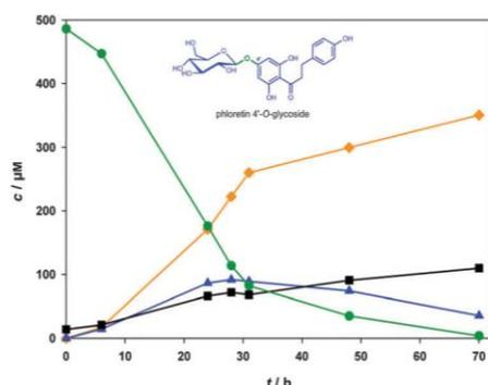
Fig. 3 Conversion of 0.5 mM phlorizin (green) by I121D mutant of *OsCGT* ( $2.5 \text{ mU mL}^{-1}$ ) in the presence of 5 mM UDP and 1 mM UDP-glucose. Further symbols: phloretin (black), nothofagin (orange), 4'-*O*-glucoside of phloretin (blue).
