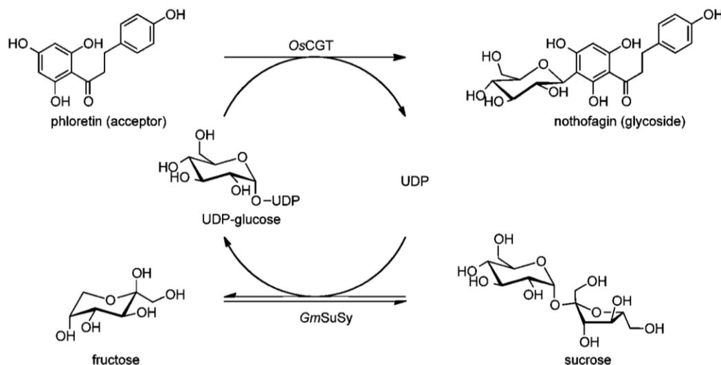
**Scheme 1.** Synthesis of nothofagin is achieved by enzymatic C-glycosylation of phloretin from sucrose via UDP-glucose. *OsCGT* and *GmSuSy* are telescoped in one pot, and the reaction proceeds in the presence of catalytic amounts of UDP. Fructose is the only by-product formed. The overall equilibrium lies far on the C-glycoside product side, driven by the reaction of *OsCGT* and the presence of sucrose in excess.
