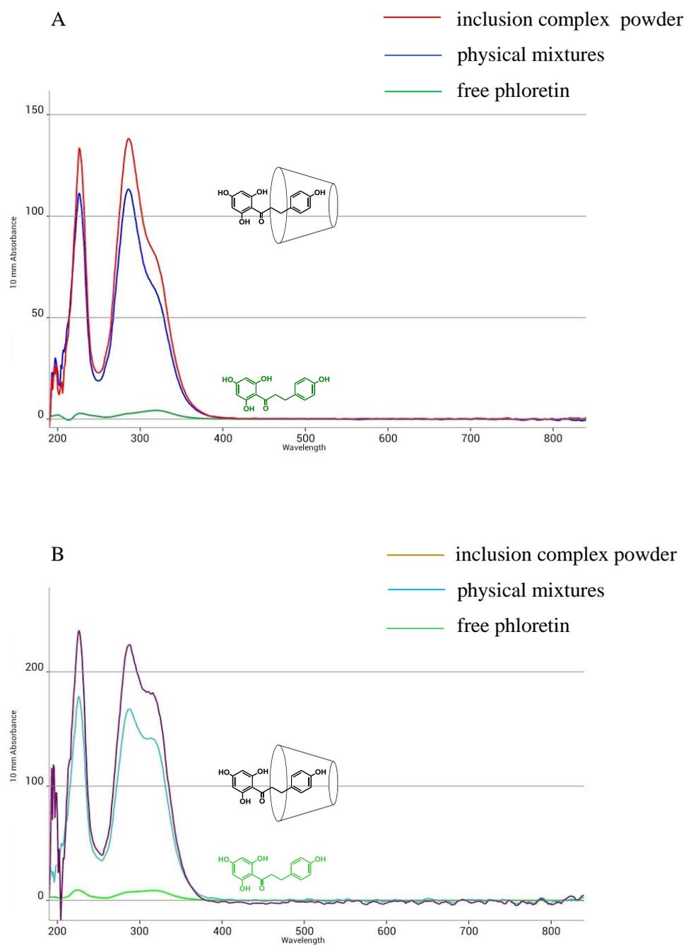
**Figure S7.** UV-VIS absorption spectra of free phloretin, phloretin/ $\beta$ -CD physical mixtures and phloretin/ $\beta$ -CD inclusion complex in A) water and B) HEPES buffer pH 7.5 showing an efficient of  $\beta$ -CD on phloretin solubility (inclusion complex > physical mixtures > free phloretin).
