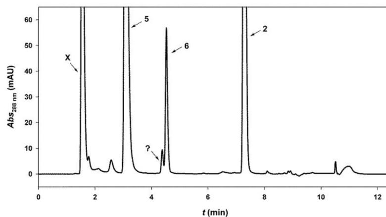
**Fig. S2** Reversed-phase C-18 HPLC-analysis of a mixture of glucosylations of **2** by *Pc*OGT and *Os*CGT I121D clearly shows that the minor product of the *Pc*OGT reaction (?) is distinct from confusoside (**6**), formed by the *Os*CGT variant.
