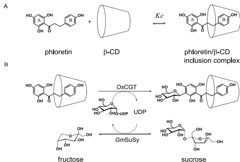
**Scheme 3.** A) Complex formation of phloretin with  $\beta$ -CD (1:1). B) Biocatalytic synthesis of nothofagin with UDP-glucose regeneration process catalyzed by *OsCGT* and *GmSuSy* in the presence of catalytic amounts of UDP.
