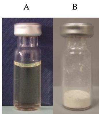
**Figure S11.** A) Aqueous solution containing 44 mM nothofagin for application on reversed phase C18 column and B) nothofagin powder as obtained after purification and lyophilization.
