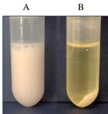
**Figure S10.** Conversion reaction of phloretin/ $\beta$ -CD inclusion complex (50 mM phloretin) (A) before adding  $5 \text{ U mL}^{-1}$  *OsCGT* and  $1 \text{ U mL}^{-1}$  *GmSuSy* and (B) after adding enzymes and incubating at  $30 \text{ }^{\circ}\text{C}$  and 20 rpm for 18 h.
