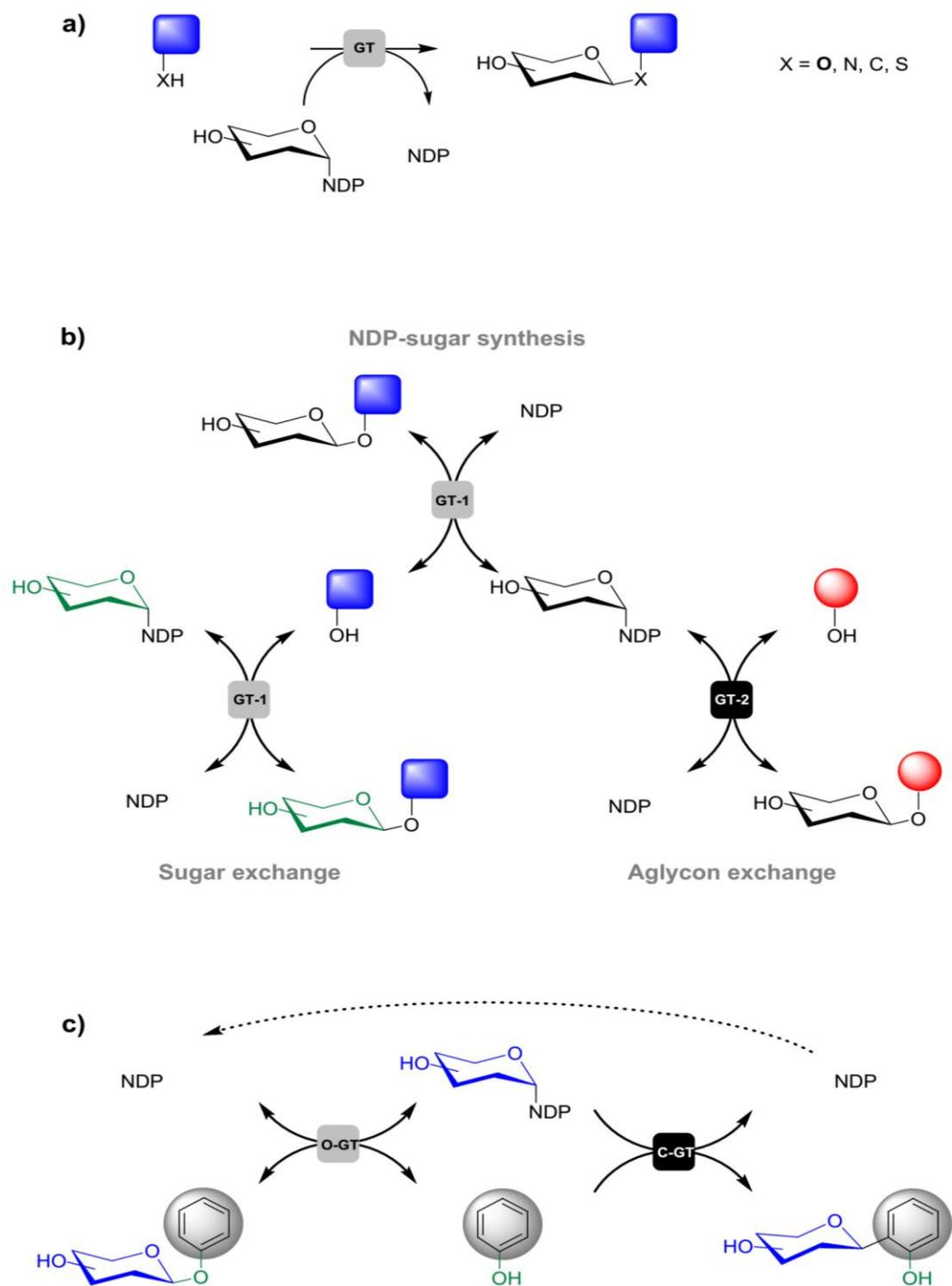
**Scheme S1** Natural product glycosylations through a canonical glycosyltransferase reaction (a), two-step exchange processes exploiting a suitable glycosyltransferase reaction in reverse direction (b), and *O*- to *C*-glycosidic bond rearrangement catalysed by complementary glycosyltransferase activities (c)
