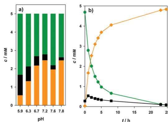
Fig. 2 Conversion of phlorizin (5 mM) via O- to C-glycosidic bond rearrangement in the presence of 2 mM UDP using 100 mU mL<sup>-1</sup> PcOGT and 50 mU mL<sup>-1</sup> OsCGT. (a) Product distribution after reaction for 5 h at different pH conditions. (b) Reaction time course at pH 7.0. Colours show phlorizin (green), nothofagin (orange), and phloretin (black).
