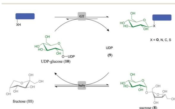
**Scheme 1** GT-catalysed cascade reaction for synthesis of natural product glucosides. Coupling of a “synthetic” GT with SuSy in one pot enables cost-effective *in situ* formation of glucosyl donor substrate **10** from **8** and catalytic amounts of **9**. End-product inhibition by **9** is obviated.
