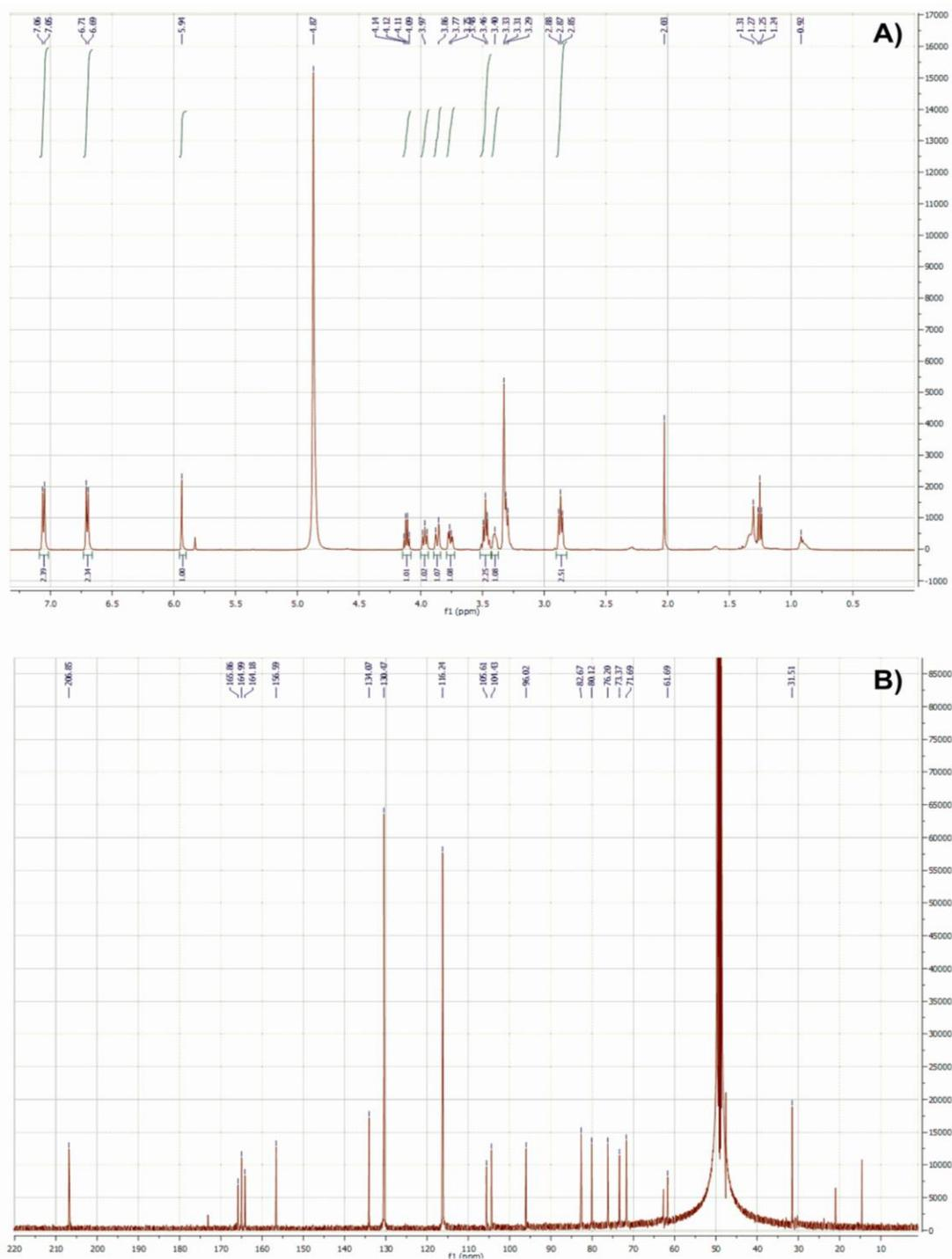
**Figure S7:**  $^1\text{H}$  A) and  $^{13}\text{C}$ -NMR B) of nothofagin after extraction with ethyl acetate from enzymatic conversion of phloretin by *OsCGT*.
