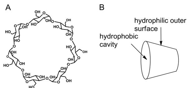
**Scheme 2.** A) Chemical structure of  $\beta$ -CD. B) Schematic drawing of CD truncated cone shape.
