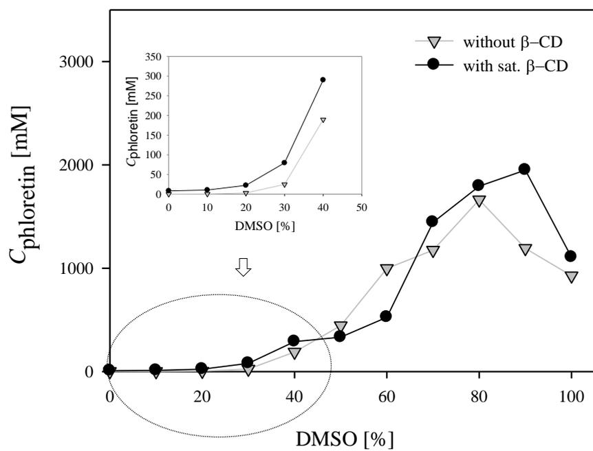
**Figure S2.** Solubility of phloretin at 30 °C using various DMSO concentrations in water in the absence and presence of excess amounts of  $\beta$ -CD.
