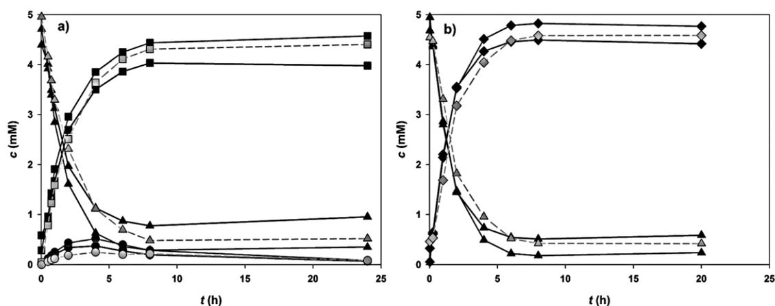
Fig. 5 Glucosylation of 5 mM **2** (triangles) at pH 7.5: black: without *GmSuSy*, 5 mM **10**; dark grey: *GmSuSy*, 5 mM **10**; light grey (dashed): *GmSuSy*, 0.5 mM **9**; (a) *PcOGT* forms **5** (squares) and an unknown compound (circles). (b) *OsCGT* I121D only produces **6** (diamonds).
