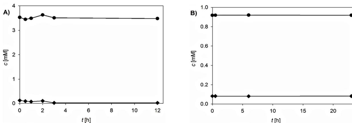
**Figure S4:** Deglycosylation of nothofagin (black) to phloretin (grey) by *OsCGT* could not be observed: A) 5 mM phloretin and 5 mM UDP-glucose were almost completely converted by  $100 \text{ mU mL}^{-1}$  *OsCGT* (not shown). When adding further 5 mM UDP (dilution) no deglycosylation of nothofagin was observed; B) Incubation of  $\sim 1 \text{ mM}$  nothofagin containing some phloretin with 1 mM UDP ( $200 \text{ mU mL}^{-1}$  *OsCGT*) did also not result in any further phloretin production.
