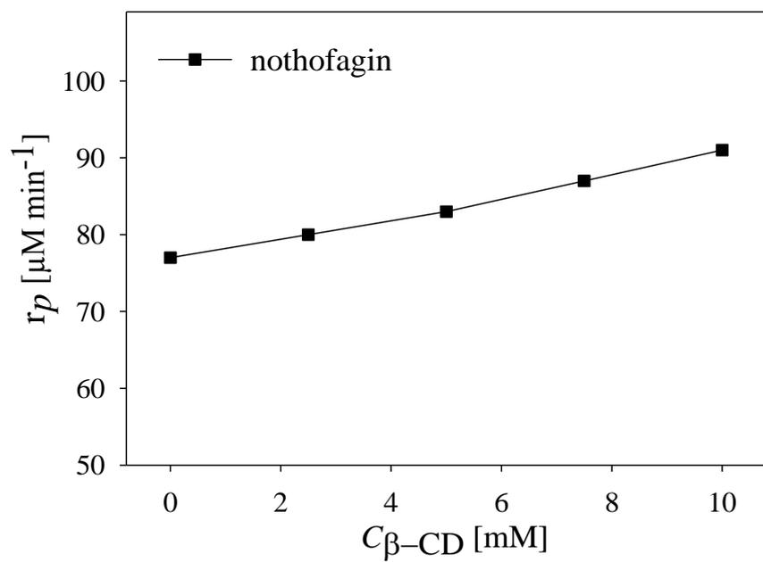
**Figure S4.** Effect of  $\beta$ -CD on *OsCGT* activity showing the nothofagin production rate increase with increasing  $\beta$ -CD concentrations.
