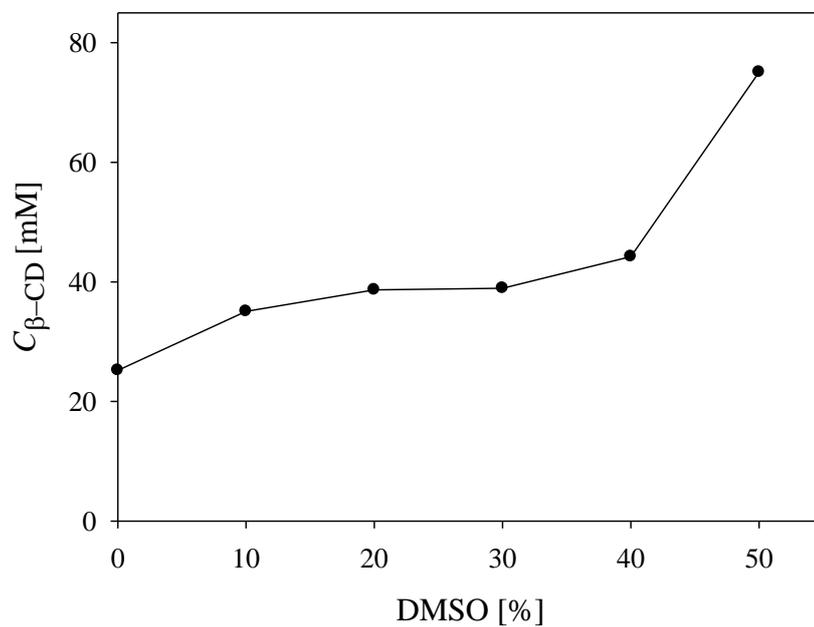
**Figure S1.** Effect of DMSO on  $\beta$ -CD solubility at 30 °C in water. The  $\beta$ -CD solubility increased at elevated DMSO concentration. It was slowly increasing from 0% to 40% DMSO (25 - 44 mM  $\beta$ -CD).  $\beta$ -CD solubility in 50% DMSO was ~1.7-fold higher than 40% DMSO.
