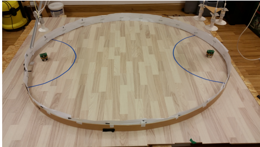
Figure 4.10.: The figure shows the setup of the social seed. Left: local optimum area with a social seed (immobilised robot). Right: global optimum area with a dummy robot to ensure similar circumstances of the two optima areas.
