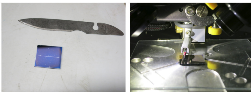
FIGURE 4.6: Determination of layer thickness by measuring height variations perpendicular to a scratch using a contact stylus profiler (EKTAK 150, Veeco).
