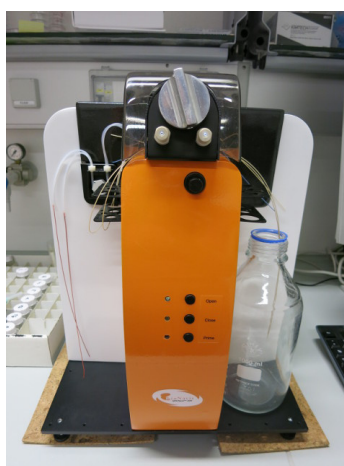
FIGURE 4.9: Surface plasmon resonance instrument (SPR Navi™ 200, BioNavis).
