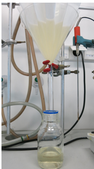
FIGURE 4.1: Filtration of hot acetic acid solutions of chitosan through a pleated filter.
