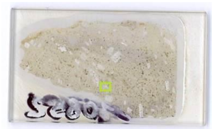
Figure B 4 Rock sample Fu9 (A) and Overview of thin section (B), in the green square even more detailed pictures were taken with transmitted and crossed nicols (see Figures 31 and 32)
