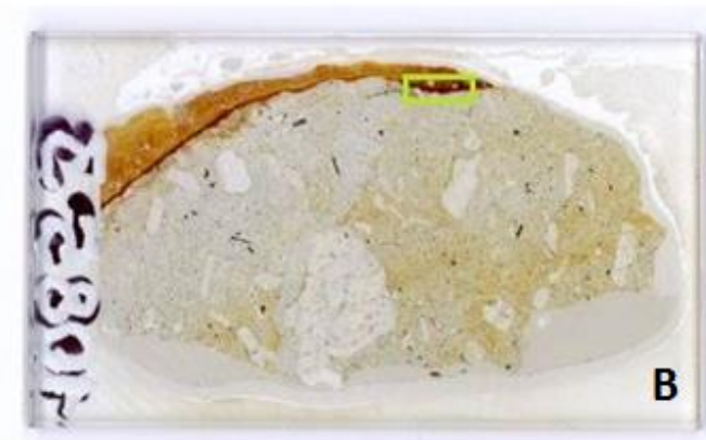
Figure B 2 Rock sample Fo9 (A) and overview of thin section (B), in the green square even more detailed pictures were taken with transmitted and crossed nicols (see Figures 28 and Figure 29)
