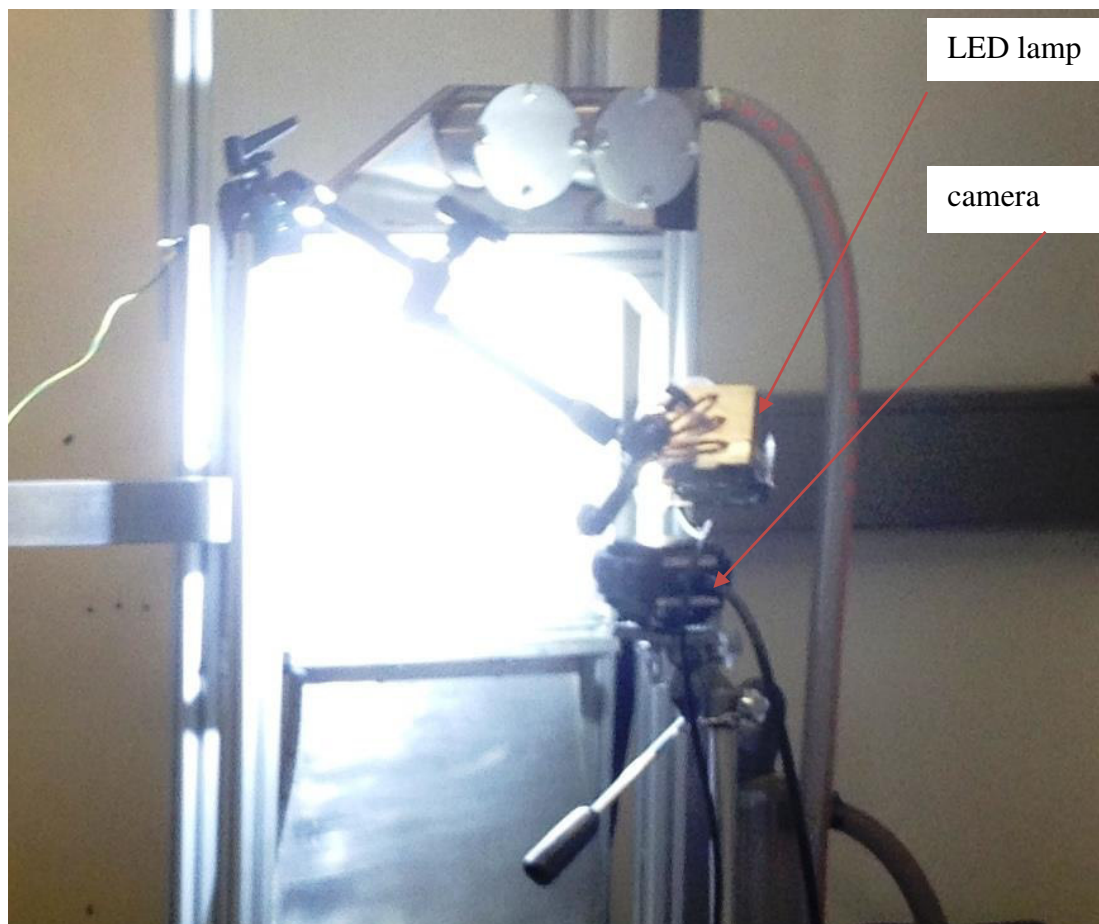
Figure 6-8: Experimental set-up for PIV image recording.
