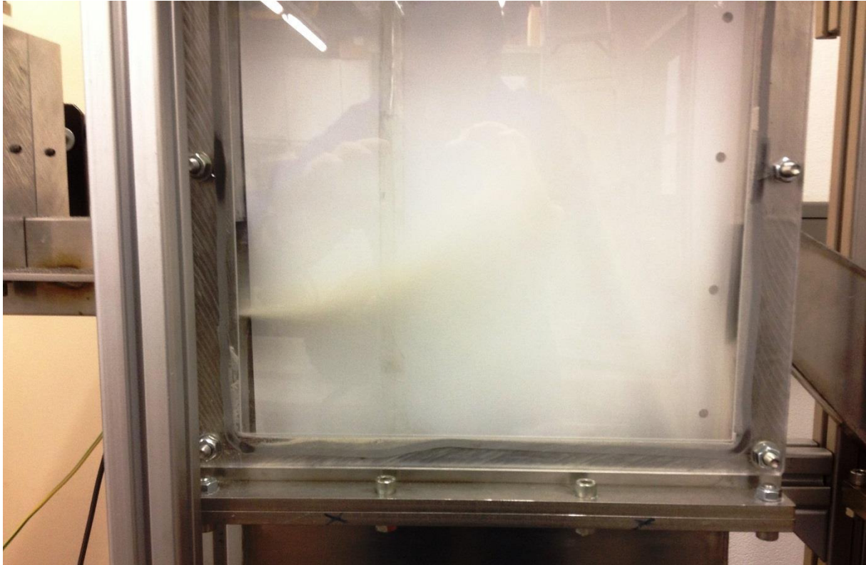
Figure 6-5: Classifying experiment for particle size distribution analysis using quartz powder with a particle size between 100 [ \mu\text{m} ] and 300 [ \mu\text{m} ], particles accelerated only mechanically by brush operated with at 24 [V].
