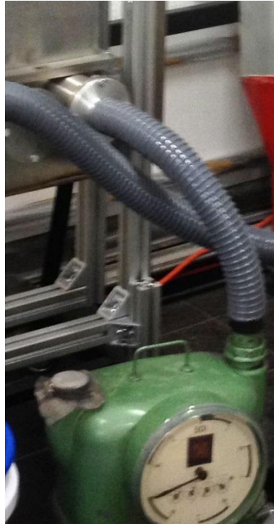
Figure 6-4: Gas meter connected to classifier air inlet.
