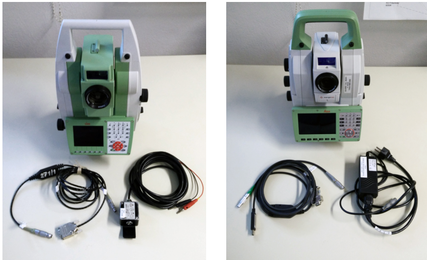
(a) Leica TS15 and Leica GEV187 (b) Leica MS60 and Leica GEV 261
