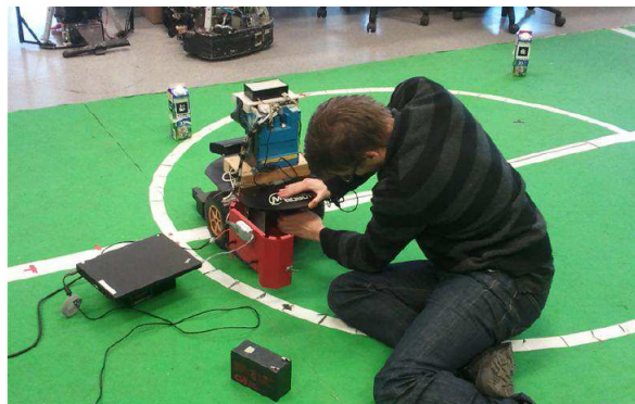
Figure 9.9.: Battery hot swap during long term robot experiment (Wolfram, 2011)
