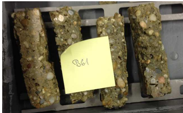
Abb.4.2: B61 (70- C 3 A-freier Zement; 10-Hüs; 15-inertes Kalksteinmehl; 5-inerter Kalkstein-MF 165)
