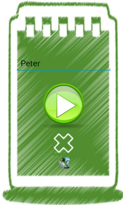
Figure 42: Start layout (part of the MainActivity) showing the name text field, Start button, Cancel button, and Setting button
