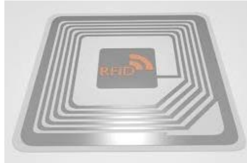
Figure 9: RFID smart label can be found in many forms and sizes. This type of tag is very popular as an alternative to QR Codes and Barcodes. 5
