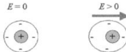
Figure 6: Electronic polarization, which shows the displacement of core and shell. 12
