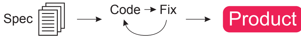
Figure 2.3.: The Code-and-Fix Model of software development contains a cycle of coding and fixing, which is repeated until someone decides it should stop. [9, Image adapted from p. 32]
