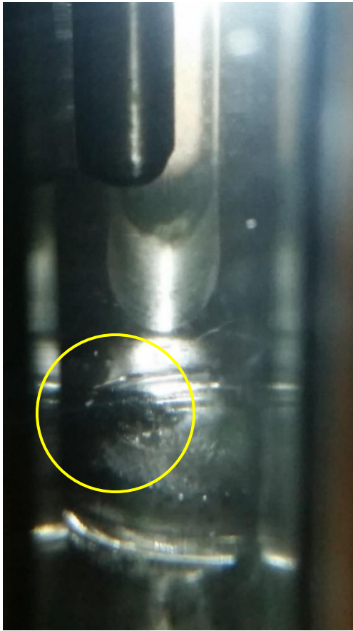
Figure 4-3 Primary copper dithizonate in scCO 2
