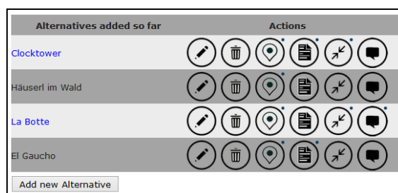
Figure 5.3.: CHOICLA: user interface for addition of decision alternatives. The dots in the upper right corner of every symbol indicate whether there is an information in this category available or not. The meaning of the used symbols is (from left to right): edit, delete, geographical information, files, links and comments .
