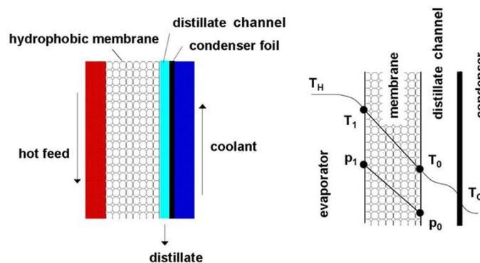
Figure 3: Scheme of membrane distillation<sup>6</sup>
