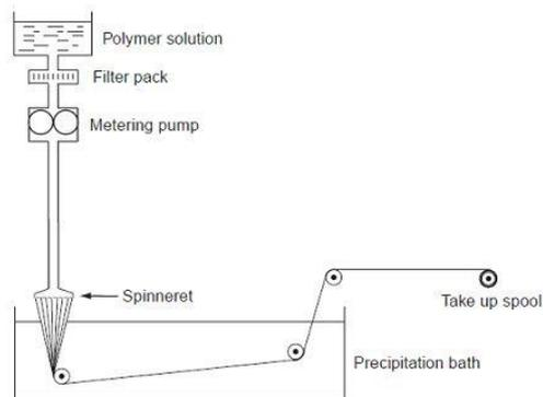
Figure 9: Dry/Wet Spinning Process<sup>18</sup>
