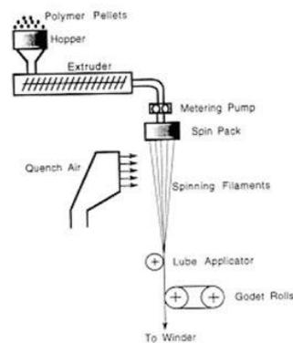
Figure 7: Melt Spinning Process <sup>16</sup>
