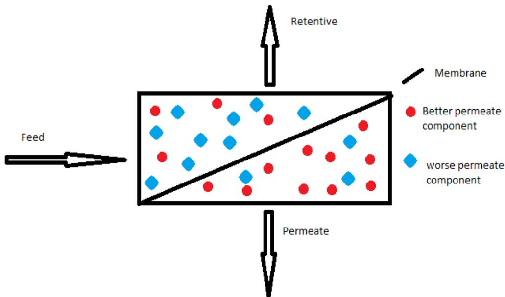
Figure 4: Membrane Separation Process
