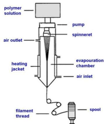
Figure 8: Dry Spinning Process<sup>17</sup>
