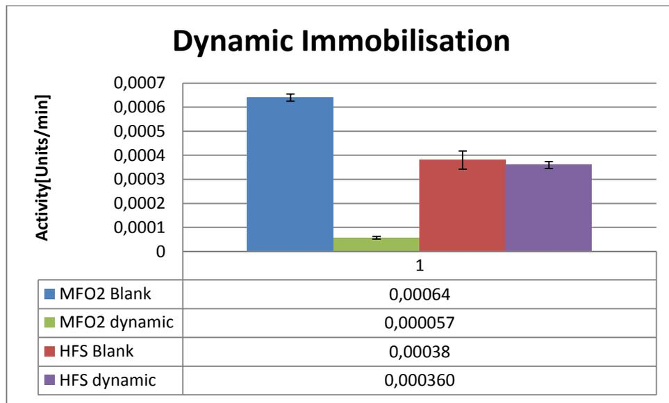
Figure 42 Comparing conventional immobilization(Blank) to dynamical immobilization
