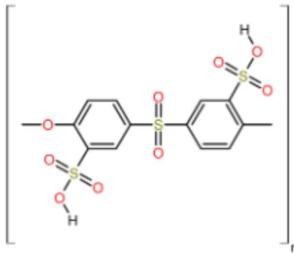
Picture 22 Structure of sulfonated polyether sulfone (S-PES)
