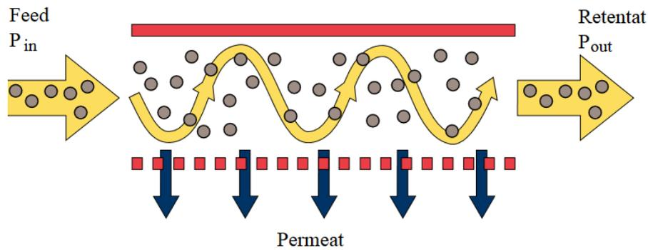
Figure 5: Cross-Flow Filtration Technique<sup>11</sup>
