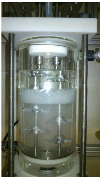
Figure S2. Settling cell (Henschke et al., 2002).
