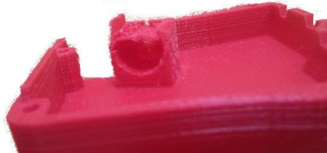
Figure 6: The 3D-printing process is not able to print big round cavities like they are needed for holding the DC-motor
