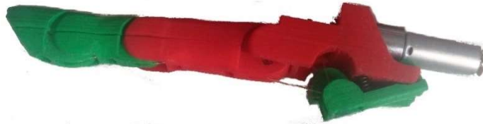
Figure 7: Example of a fully assembled phalanges II – IV. The motor is positioned at the rear of the finger.
