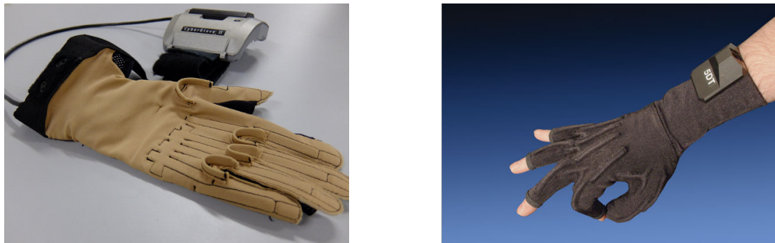
Figure 4.2.: The CyberGlove (left) and the 5DT Data Glove (CyberGlove Systems Inc, 2015; 5DT Inc, 2015)
