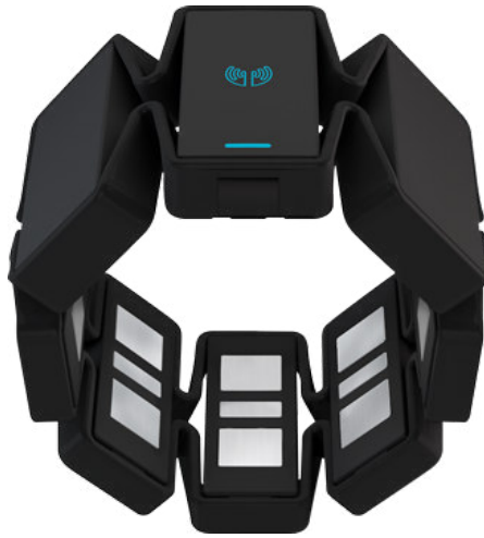
Figure 4.6.: The Myo wearable gesture and motion detection armband. (Thalmic Myo, 2016)
