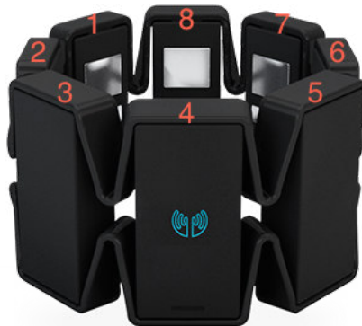
Figure 5.9.: The numbering of Myo's EMG sensors (Thalmic Myo, 2016). The numbers correspond to the indices in the data array provided by the LSL application.
