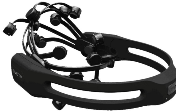
Figure 4.3.: The Emotiv EPOC wireless EEG headset (Emotiv, 2015)
