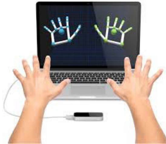
Figure 4.5.: The Leap motion controller and the hand tracking model. (Leap Motion, 2015)
