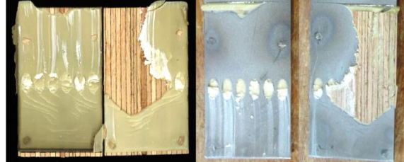
LBD-PU-SA-08 F_{\max} = 50,8 \text{ kN} Bruch = unten
