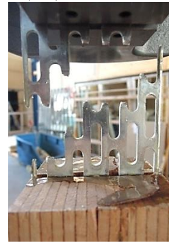
LBL-ESS-CO-02 („h“) F_{\max} = 5,8 \text{ kN}
