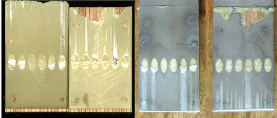
LBD-PU-SA-03 F_{\max} = 50,9 \text{ kN} Bruch = unten
