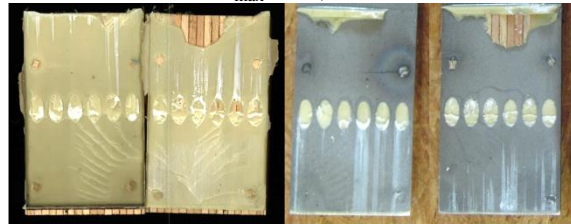
LBD-PU-SA-10 F_{\max} = 45,6 \text{ kN} Bruch = unten
