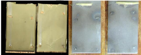
S5-PU-SA-09 F_{\max} = 40,4 \text{ kN} Bruch = unten
