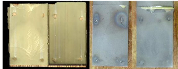
S5D-PU-SA-10 F_{\max} = 48,0 \text{ kN} Bruch = unten
