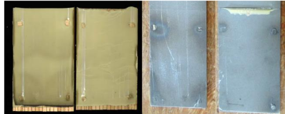
S5-PU-SA-06 F_{\max} = 33,5 \text{ kN} Bruch = oben
