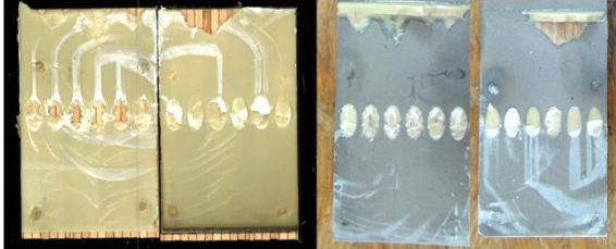
LBD-PU-SA-07 F_{\max} = 48,1 \text{ kN} Bruch = oben
