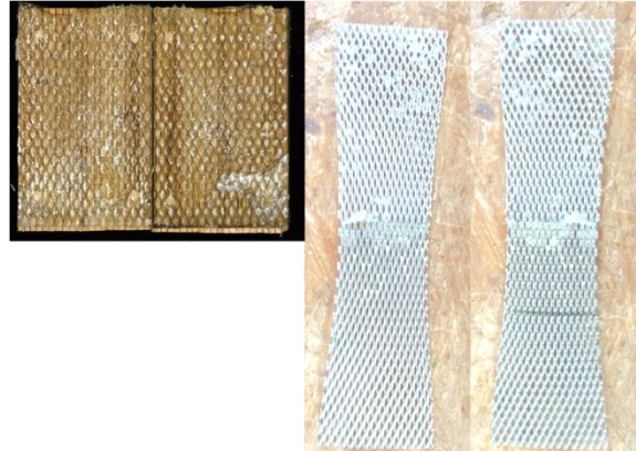
LBL-ESS-CO-02 („h“) F_{\max} = 5,8 \text{ kN}
