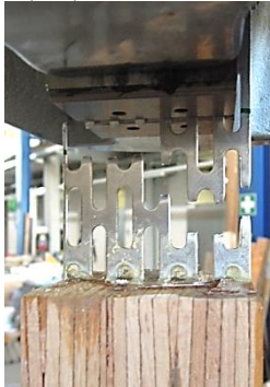
LBL-ESS-CO-01 („h“) F_{\max} = 5,9 \text{ kN}
