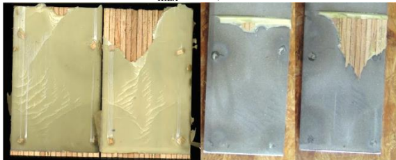
S5-PU-SA-09 F_{\max} = 40,4 \text{ kN} Bruch = unten
