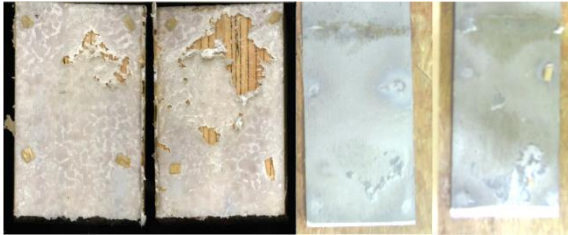
S5-HB-SA-03 F_{\max} = 30,3 \text{ kN} Bruch = oben
