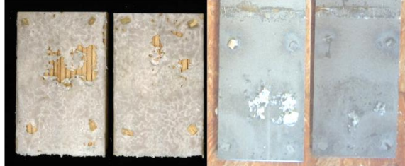
S5-HB-SA-06 F_{\max} = 25,4 \text{ kN} Bruch = unten
