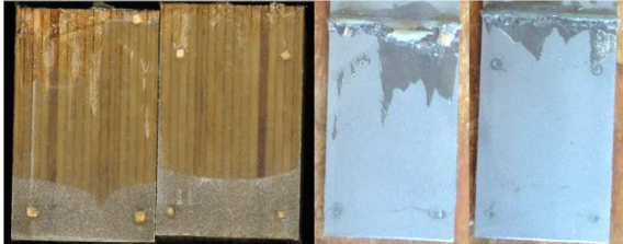
S5-COQ-SA-01 F_{\max} = 65,2 \text{ kN} Bruch = unten
