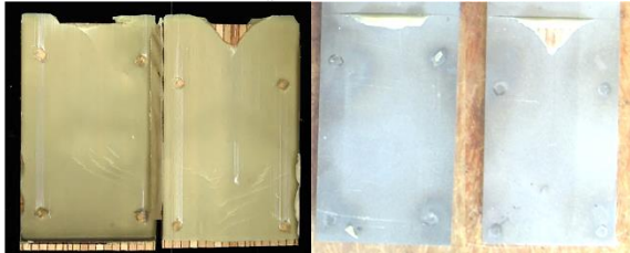
S5-PU-SA-05 F_{\max} = 38,0 \text{ kN} Bruch = unten
