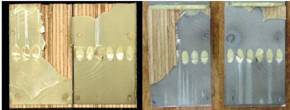
LBD-PU-SA-09 F_{\max} = 49,3 \text{ kN} Bruch = unten
