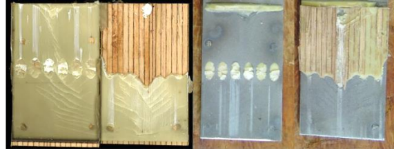
LBD-PU-SA-06 F_{\max} = 47,3 \text{ kN} Bruch = oben
