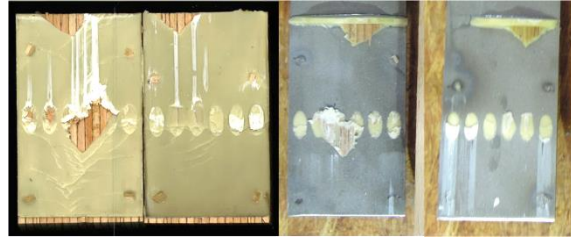
LBD-PU-SA-04 F_{\max} = 50,3 \text{ kN} Bruch = oben
