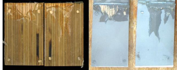
S5- CO-SA-04 F_{\max} = 51,6 \text{ kN} Bruch = unten
