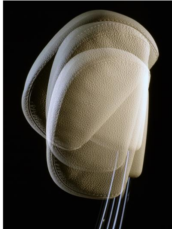
FIGURE 29 DAIMLER NECK PRO - ACTIVE REUSABLE ANTI-WHIPLASH HEAD RESTRAINT SYSTEM (DAIMLER AG, 2012)
