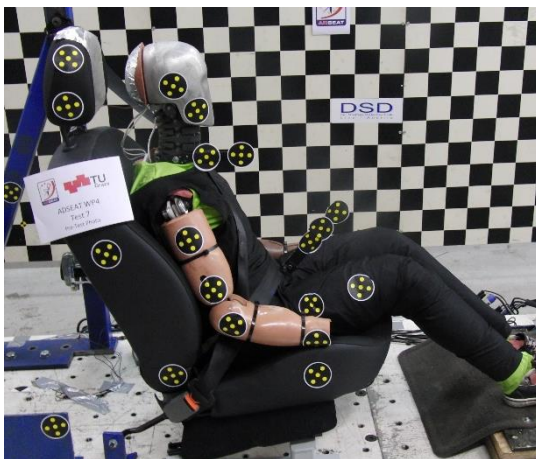
FIGURE 37 SETUP OF TEST NO. TUG11007 BIO RID 50F IN SEAT A
