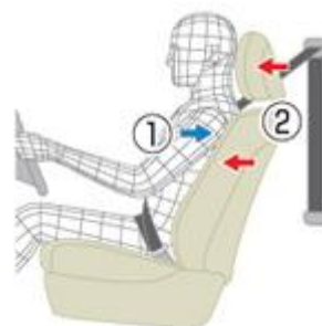
FIGURE 32 TOYOTA WIL CONCEPT PRINCIPLE FUNCTIONALITY (TOYOTA MOTOR CORPORATION, 1995-2015)
