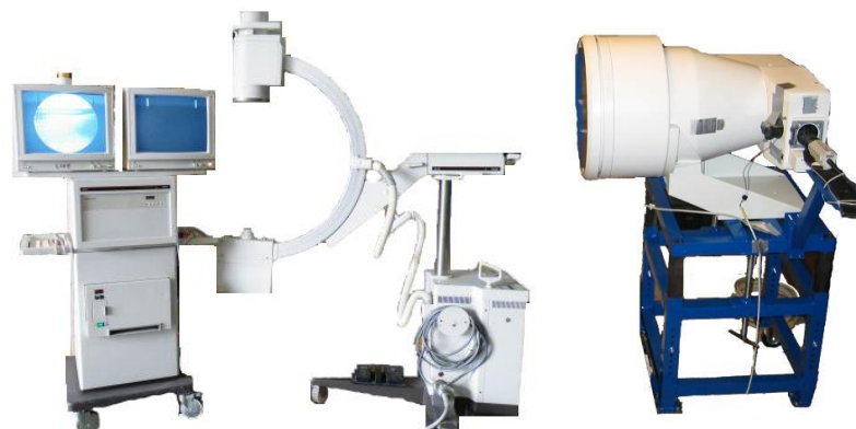
FIGURE 45 PMHS C-ARM X-RAY SYSTEM WITH IMAGE INTENSIFIER.
