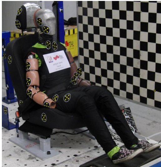
FIGURE 36 OVERVIEW OF THE MODIFIED BIO RID 50F IN SEAT A
