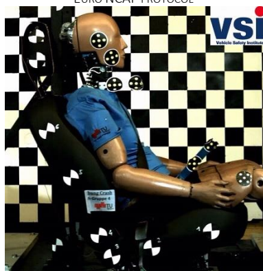
FIGURE 56 OOP SETUP OF THE OOP 4 TEST CONFIGURATION, REFERENCE ACCORDING TO THE EURO NCAP PROTOCOL
