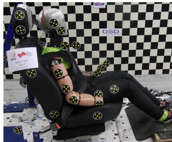
FIGURE 38 SETUP OF TEST NO. TUG11008 BIO RID 50F IN SEAT A
