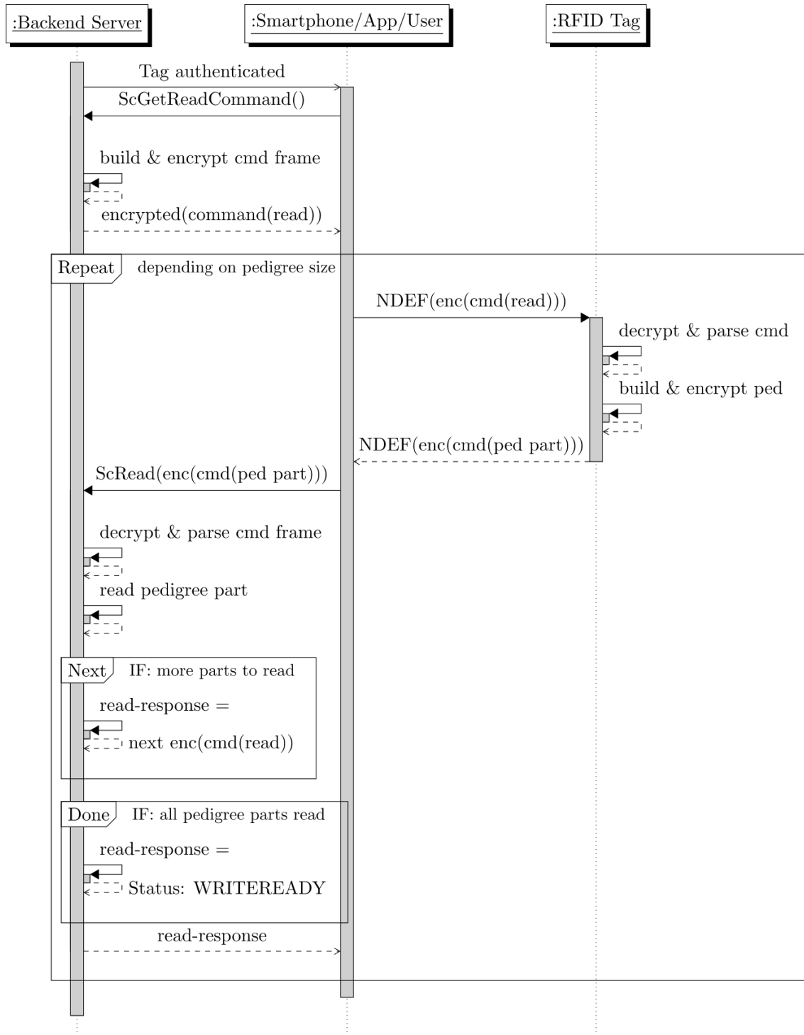
Figure 3.15: Detailed Sequence Diagram of the Read Operation
