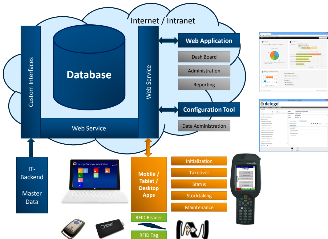
Figure 3.3: Architectural Overview of detego SURVEYOR (developed by Enso Detego GmbH)
