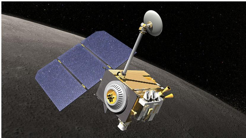
Figure 5.1: Artist concept of the Lunar Reconnaissance Orbiter (©NASA). The dimension of the main spacecraft bus is approximately  $1.3 \times 1.4 \times 2.2$  m. Several scientific instruments are attached to the bus along with a single solar array and a high gain antenna.
