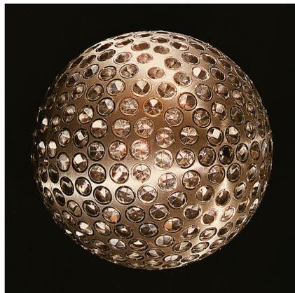
Figure 4.1: Illustration of the LAGEOS-1 satellite. Its surface is covered by 426 corner cube reflectors (image credit: NASA).
