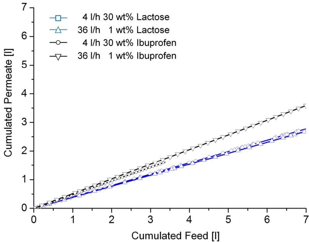
Figure 7 Cumulative permeate flow over cumulative feed flow. The gradients for all runs, as listed in Table 1, show a constant material-dependent slope. For reasons of clarity, only two extreme cases are shown for each model substance (only every 80<sup>th</sup> data point plotted)
