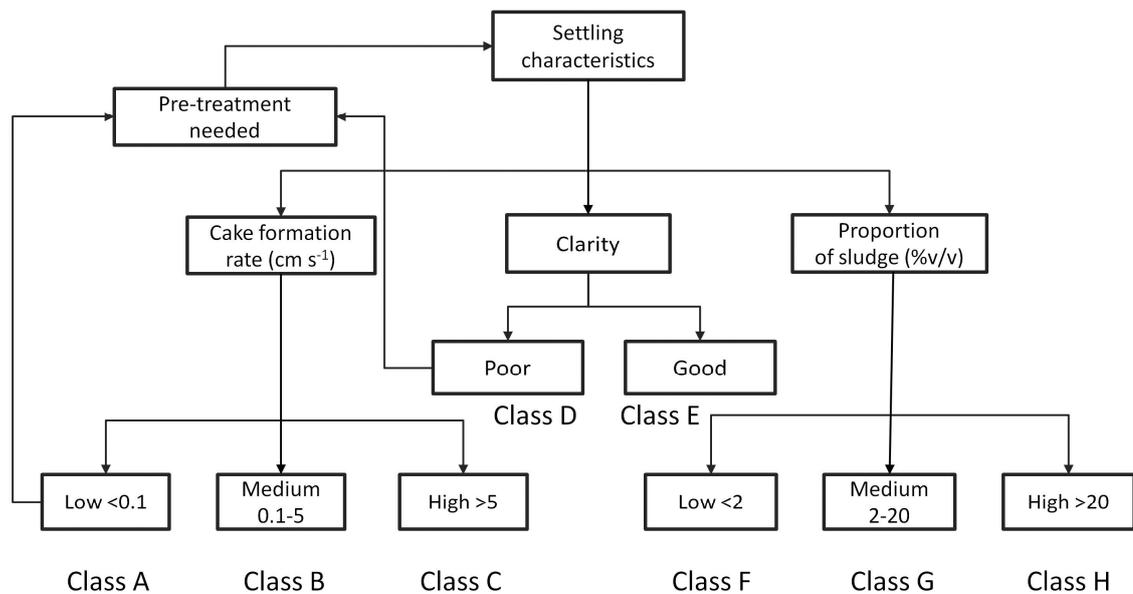
Figure 4 Decision tree as structural approach to select a generic equipment class based on settling characteristics [23]
