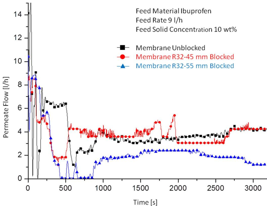
Figure 14 Permeate flow rate for partially blocked and unblocked membranes (only every 50<sup>th</sup> data point plotted)
