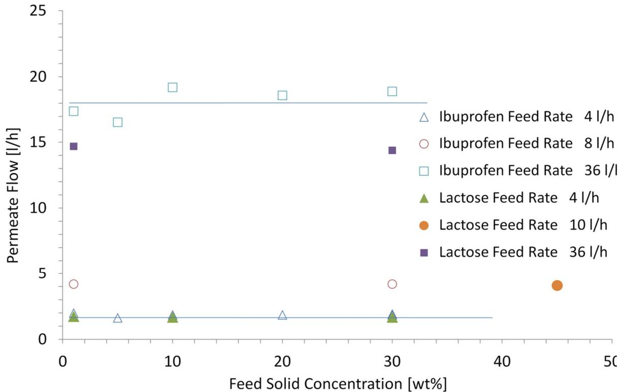
Figure 9 Permeate flow over feed solid concentration for lactose and Ibuprofen
