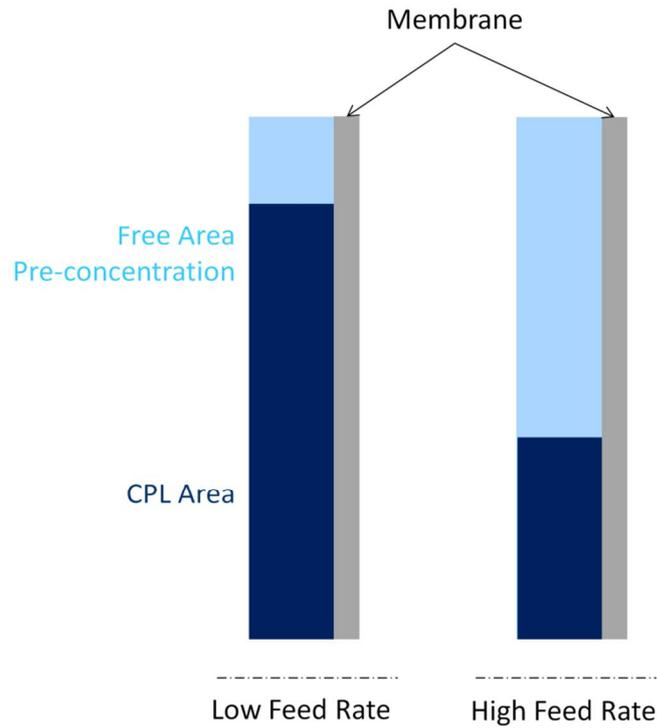
Figure 12 Schematic of the underlying effects concerning CPL buildup
