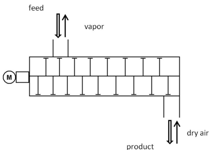
Figure 4 Schematic of the paddle dryer from Hosokawa Micron
