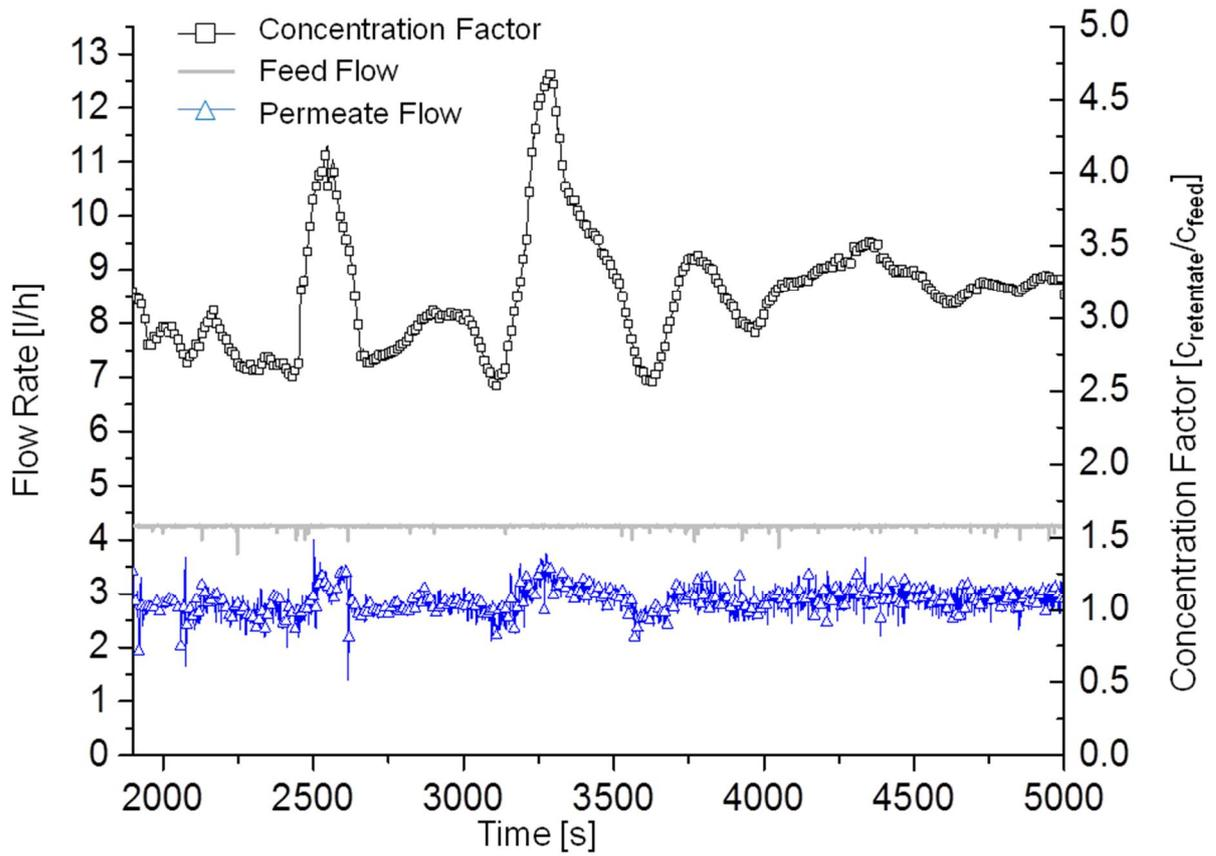
Figure 5 Experimental results for the vacuum-enhanced open operation mode with lactose (only every 10<sup>th</sup> data point plotted). The large fluctuations in the permeate flow and in CF from 2000 to 4000 s result from variations in the vacuum pump speed. During this time span, the vacuum pump speed was manually manipulated to maximize CF while avoiding transgression of maximal solid concentration levels as defined by a ramp-up test
