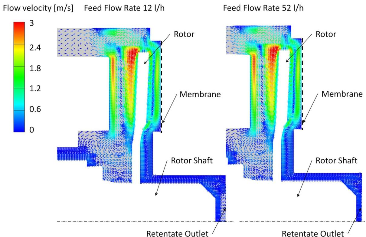
Figure 11 Influence of the feed flow rate on the velocity profile in the CFF. The axis of rotation is shown as dashed line
