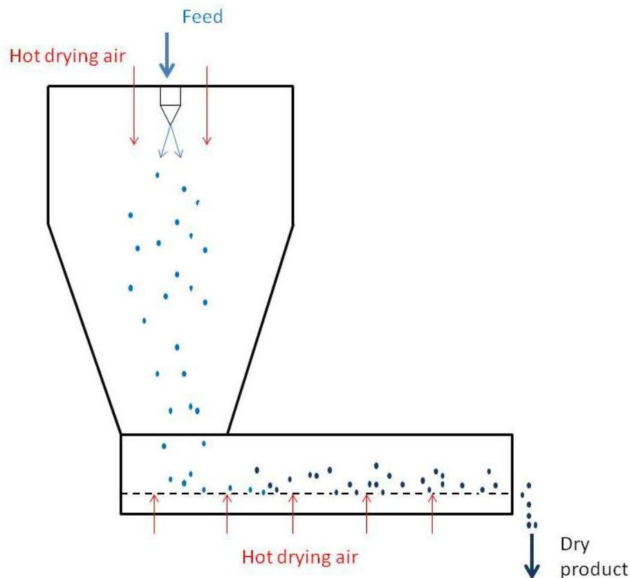
Figure 5 Schematic of a spray dryer with integrated fluid bed
