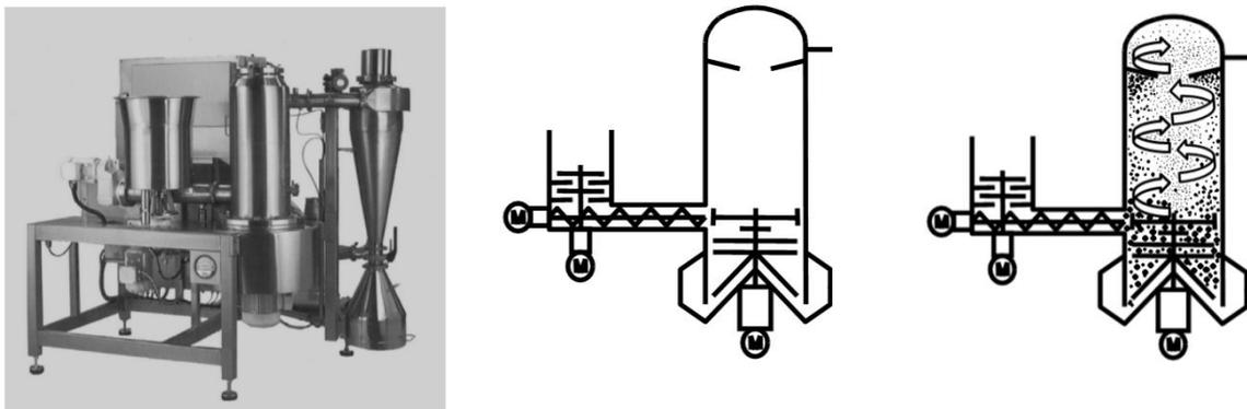
Figure 3 Main components and working principle of a spin flash dryer [45]
