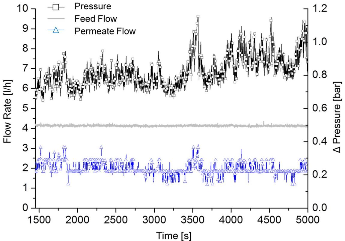
Figure 8 Experimental results for pulsation operation mode with Ibuprofen (only every 10<sup>th</sup> data point plotted)
