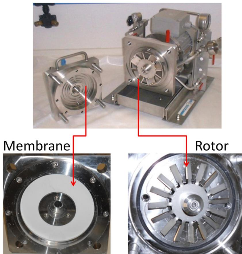
Figure 1 Pictures of the CFF (Dynotest® by Bokela GmbH) with rotor and ceramic membrane
