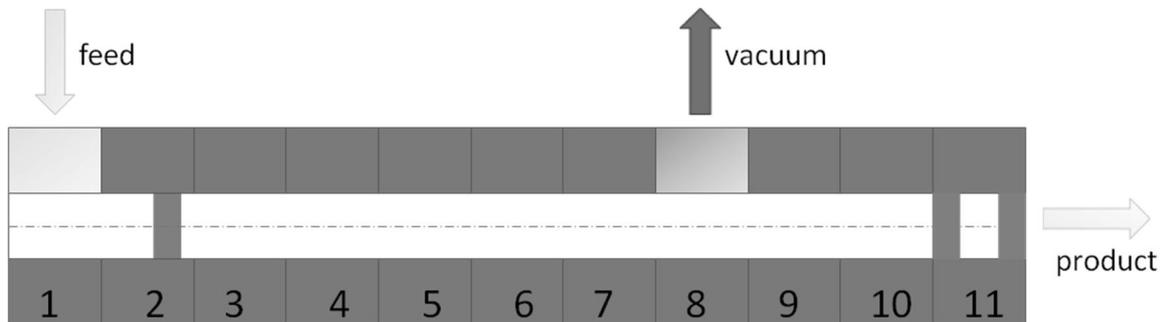
Figure 6 Housing blocks and selected screw elements for screw configuration 1 with a sealed end used for vacuum drying and counter- or co-current drying. Flow streams are indicated for vacuum drying
