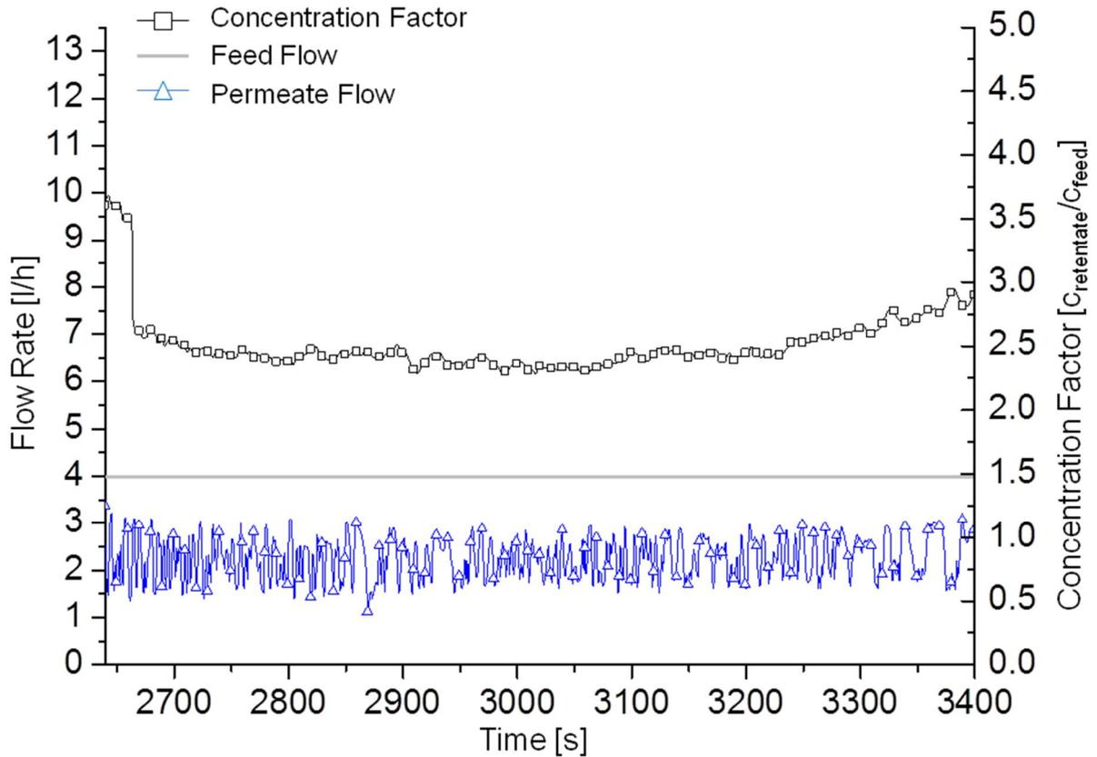
Figure 6 Experimental results for vacuum-enhanced open operation mode with Ibuprofen (only every 10<sup>th</sup> data point plotted)
