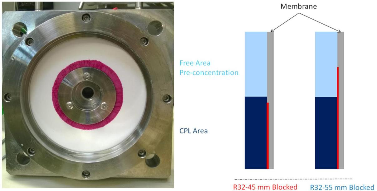
Figure 13 Partially blocked membrane used during verification runs and schematic of the CPL buildup in correspondence to blocked membrane area. With a blocked membrane, actual CPL buildup might not occur as indicated due to the absence of flow through the blocked membrane area
