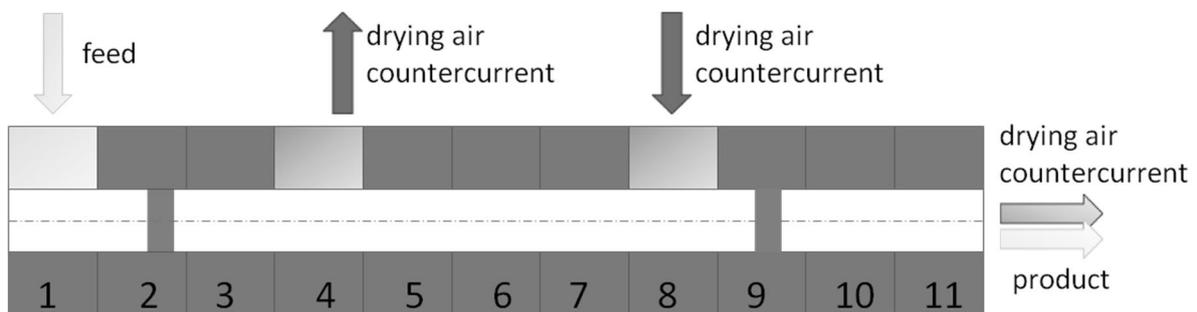
Figure 8 Housing blocks and selected screw elements for screw configuration 3 with a clogged end used for counter- or co-current drying. Flow streams are indicated for countercurrent drying
