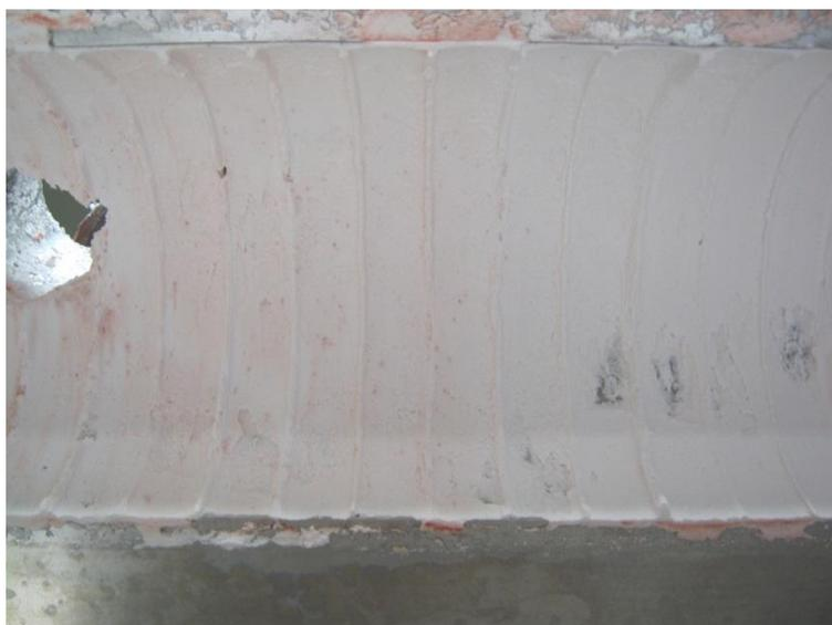
*Figure 11 Wet pasty phase just past the feed port after adding iron oxide as a colorant to determine the residence time distribution*
