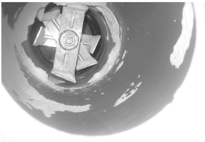
Figure 9 Deposit build-up during start up of Ibuprofen drying
