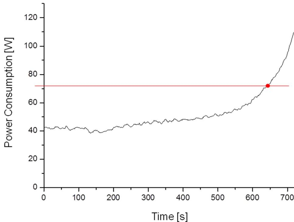
Figure 4 Ramp-up test for lactose to determine rotor load setpoint
