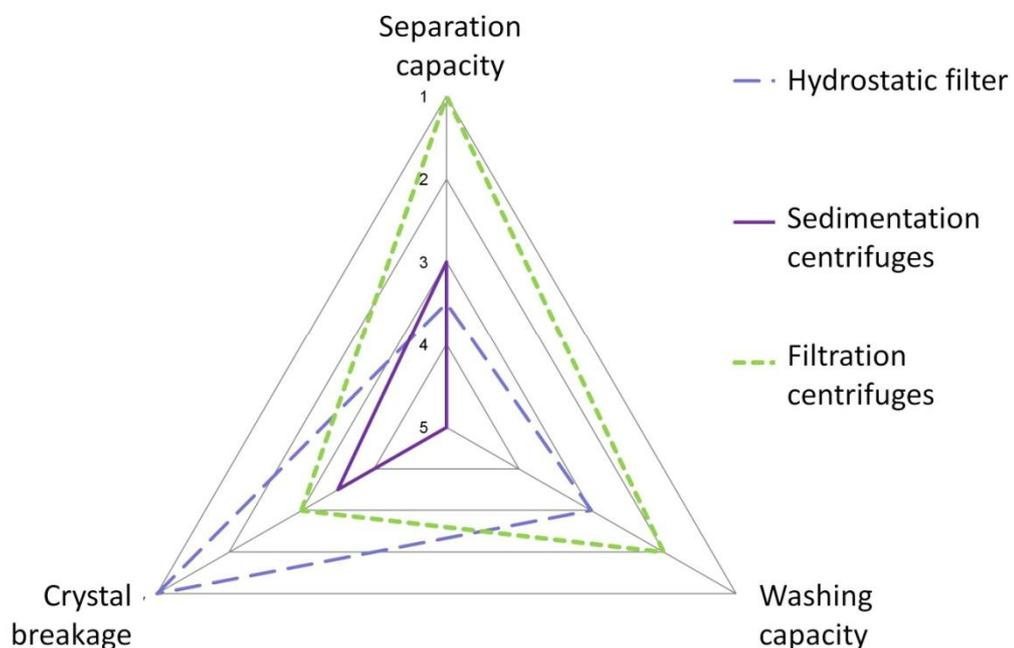
Figure 3 Graphical illustration of the information presented in a ranked table. Three technologies are evaluated according to their performance concerning separation capacity, risk of crystal breakage and washing capacity (one...very good, five...insufficient)
