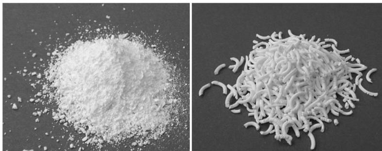
Figure 12 From left to right: Ibuprofen flakes produced with screw configuration 1, extruded Ibuprofen strands produced via vacuum drying
