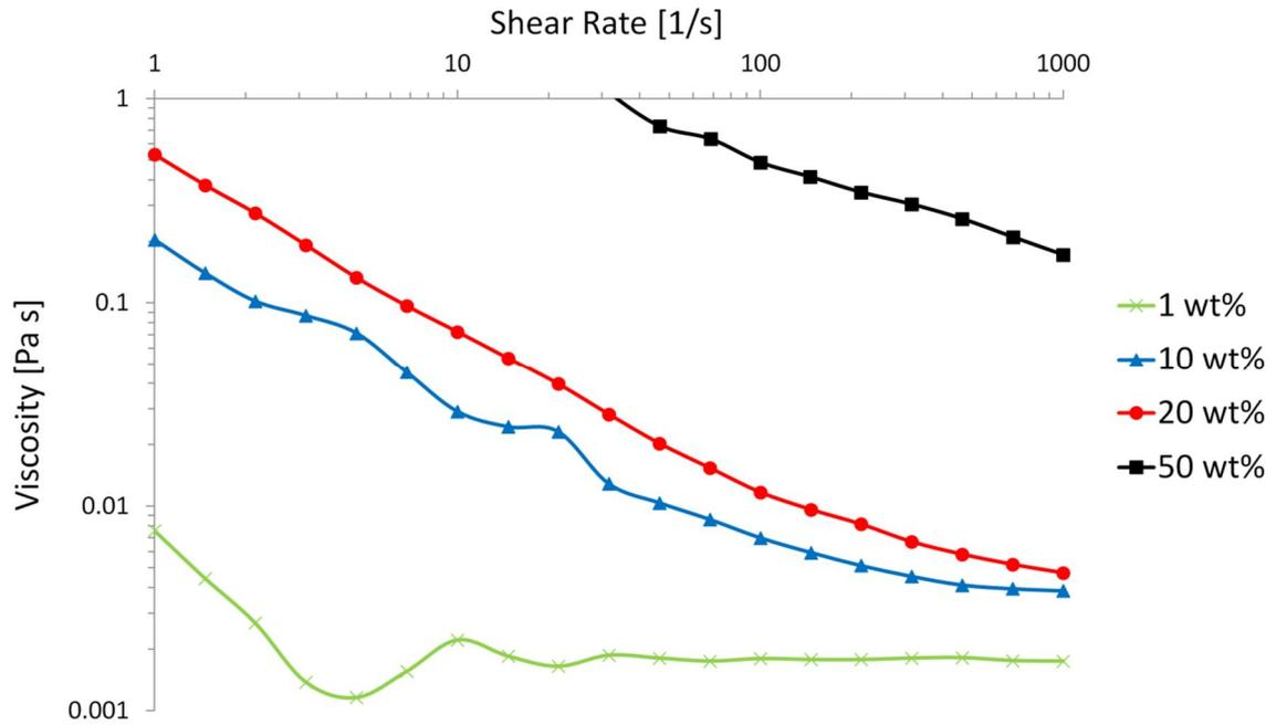
Figure 6 Viscosity over shear rate for Ibuprofen suspensions in double logarithmic scale
