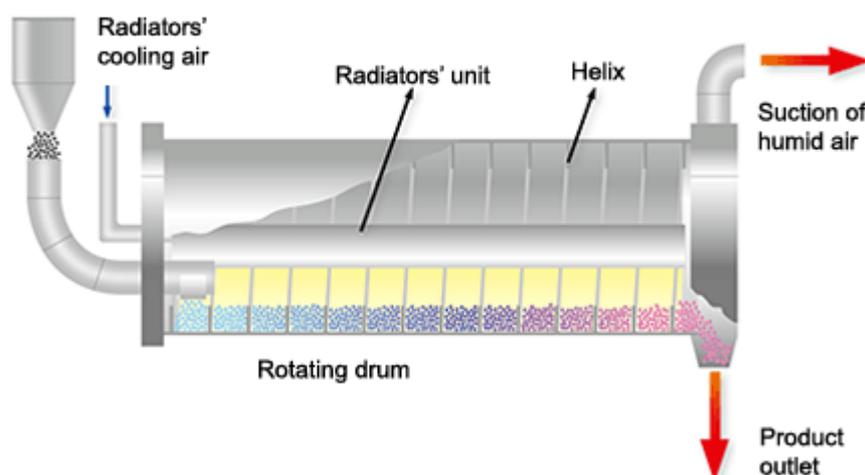
Figure 8 Schematic of an Infrared rotary drum process [60]
