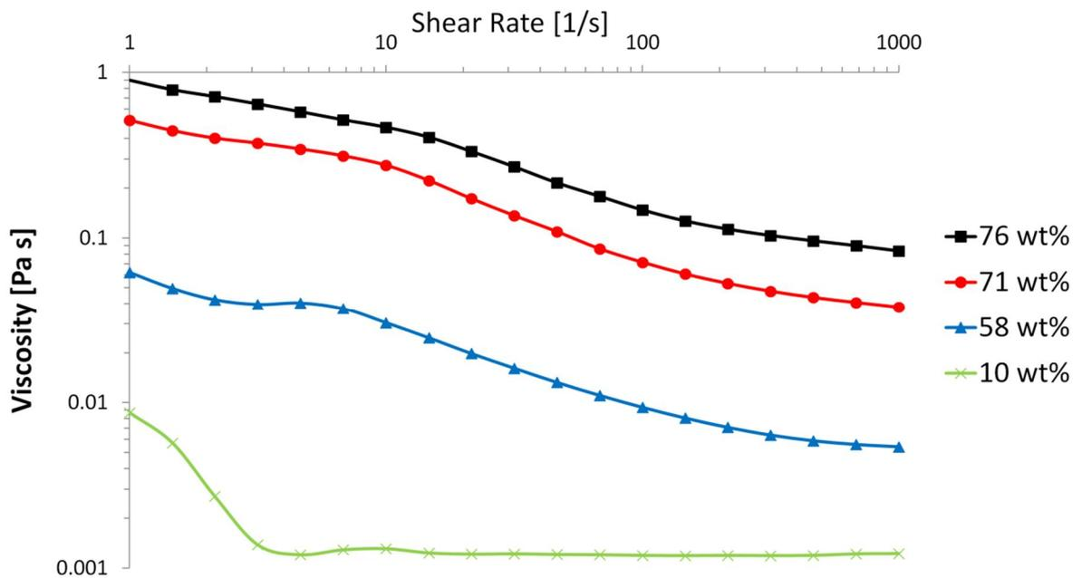
Figure 5 Viscosity over shear rate for lactose suspensions in double logarithmic scale
