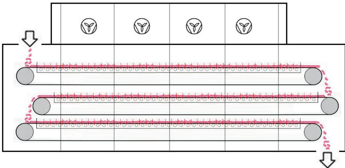
Figure 7 Schematic of a belt dryer with multiple conveyor belts for large throughputs and long residence time
