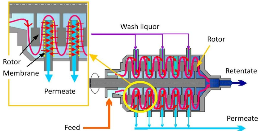
Figure 2 Modular multi-chamber dynamic cross-flow system Bokela DYNO® Filter [30]
