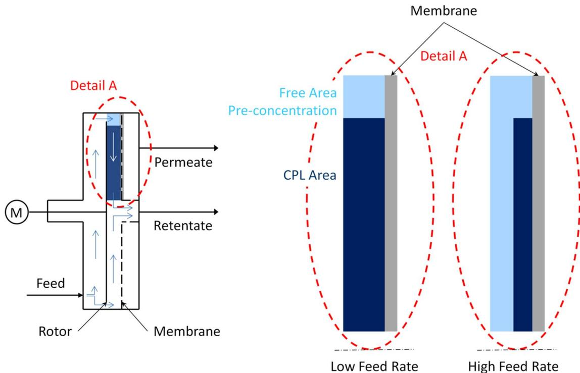
Figure 10 Schematic of the filter system and of a possible CPL structure suggesting a variation of CPL thickness in dependence of the feed rate. The axis of rotation is shown as dashed line. Suspension flow occurs from the outside towards the inside over the membrane as shown. The assumption is that a certain region outside (due to high velocity of the rotor) is free of a CPL
