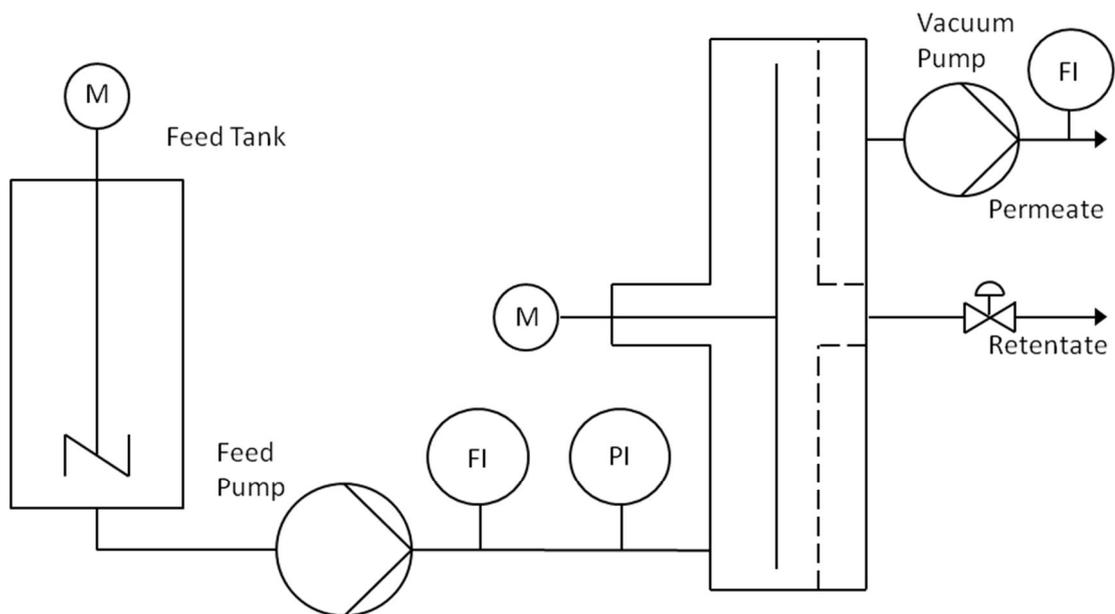
Figure 2 Schematic of the filtration setup
