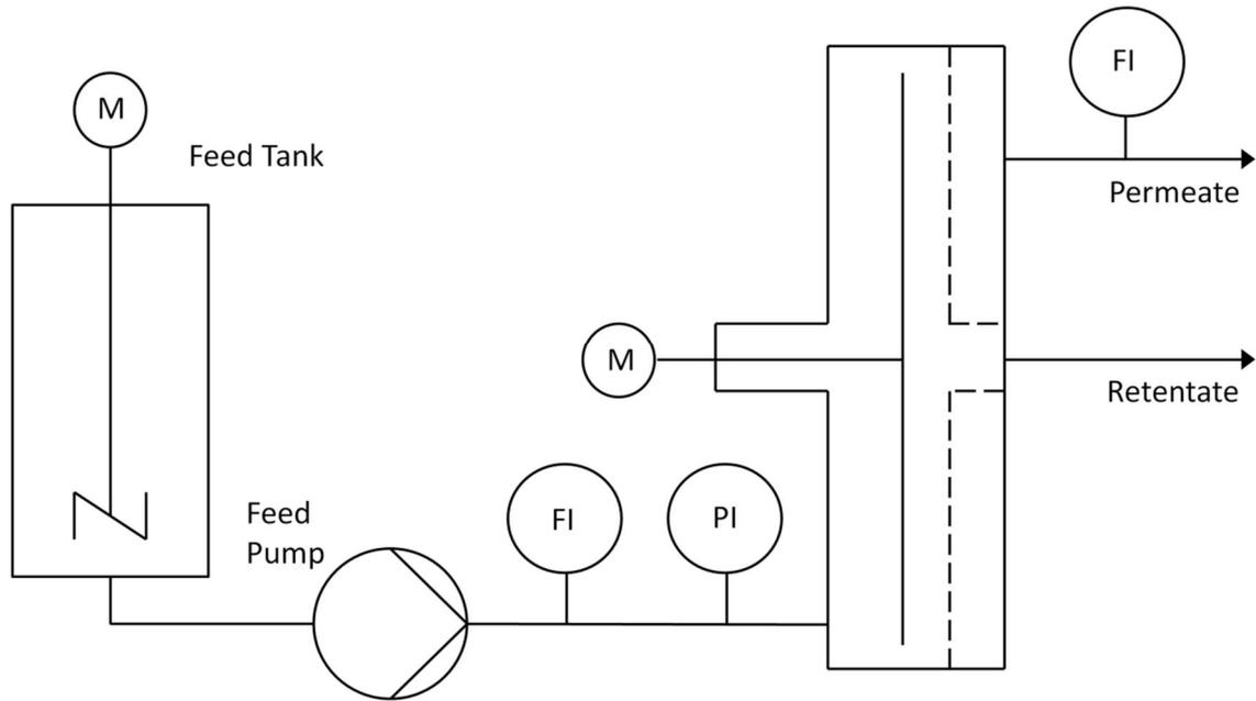
Figure 2 Schematic filtration setup
