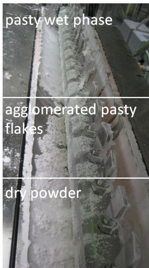
Figure 10 Three sections formed during drying with the paddle dryer. The lower half of the heated tube is shown. Each paddle can be inclined individually. The picture shows drying of Ibuprofen
