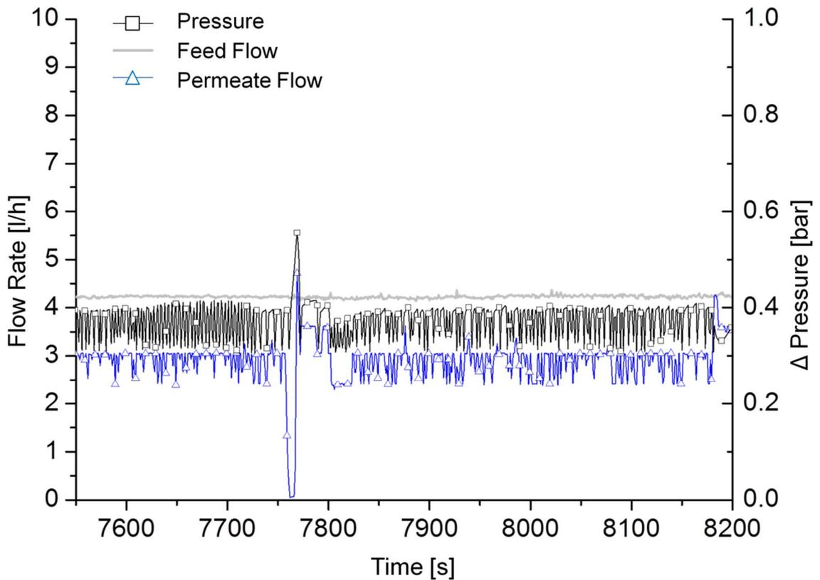
Figure 7 Experimental results for pulsation operation mode with lactose (only every 10<sup>th</sup> data point plotted) The peak measured at 7760 seconds results from a short term material congestion at the retentate valve. However, the subsequent pressure rise sufficiently removed the congestion
