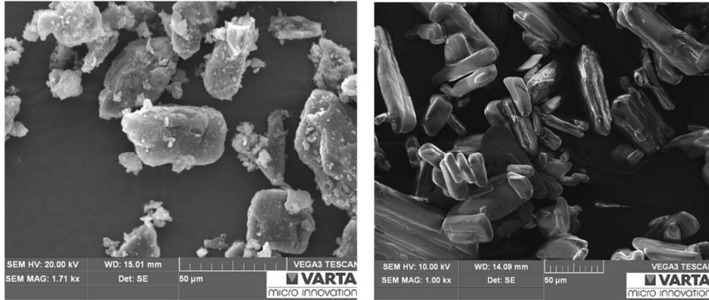
Figure 4 SEM images of lactose (left) and Ibuprofen (right)
