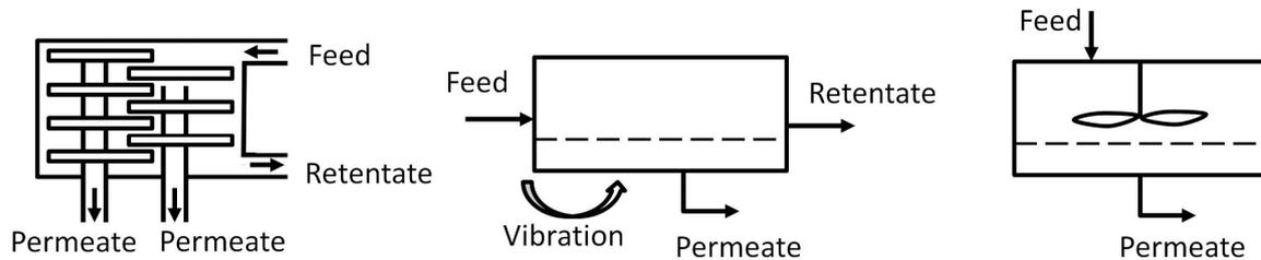
Figure 1 Dynamic cross-flow filtration principles (from left to right): rotating cylindrical systems, rotating disk systems, vibrating systems, systems with integrated stirrers [18], [28]
