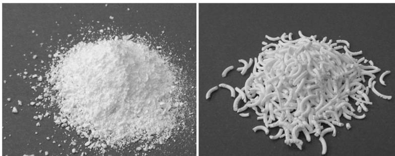
Figure 12 From left to right: Ibuprofen flakes produced with screw configuration 1, extruded Ibuprofen strands produced via vacuum drying
