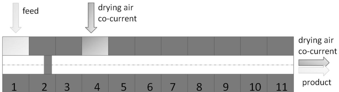
Figure 7 Housing blocks and selected screw elements for screw configuration 2 with an open end used for counter- or co-current drying. Flow streams are indicated for co-current drying
