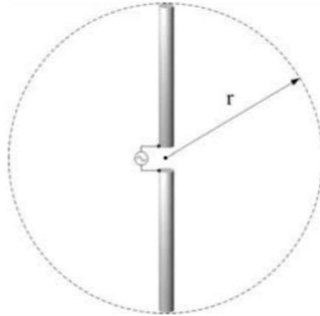
Figure 3: Dipole antenna [3]
