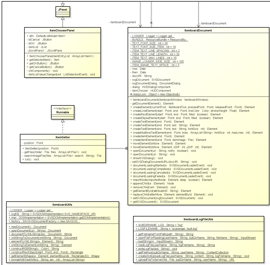
Figure 4.21.: Simplified class diagram of the client side of the Itemboard module - Part 2
