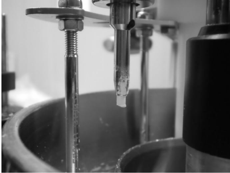
Fig. 1: Piston blocking of the 3.4 mm dosator: Extensive pre-compression of the powder occurred due to a 1:5 compression ratio between dosing chamber length and powder layer depth. A very hard plug was formed, which could not be ejected by the piston.
