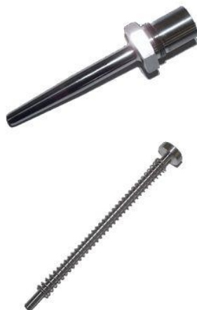
Figure 8: Dosator filling mechanism: Lab scale machine dosator (MG2, Italy)
