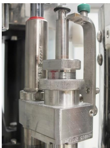
Figure 5: Picture of the caliper used to fix the position of the piston in the nozzle (and hence the size of the dosing chamber).
