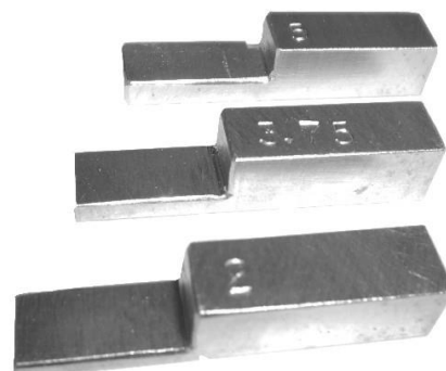
Fig. 4: Gauge to adjust the dosing chamber length
