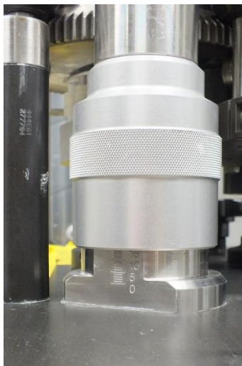
Figure 6: Picture of the caliper used to fix the depth of powder bed in the bowl (located at the base of the shaft that controls the vertical position of the bowl).
