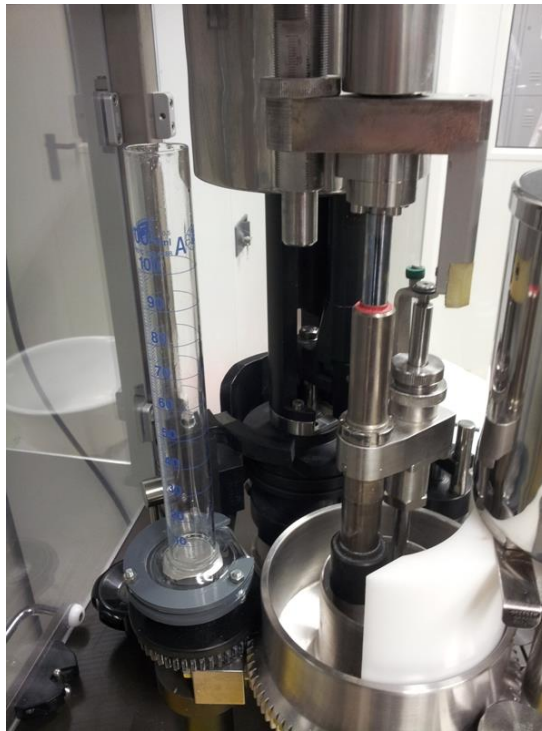
Figure 2: A graduated cylinder fixed with a clamp to the knob located on a rotating disc that is intermeshing with the teeth of the powder bowl.
