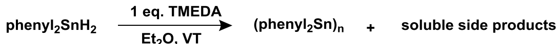
Scheme 80: Dehydrogenative coupling of \text{phenyl}_2\text{SnH}_2 leading to an insoluble polystannane (\text{phenyl}_2\text{Sn})_n and soluble side products (VT= variable temperature).
