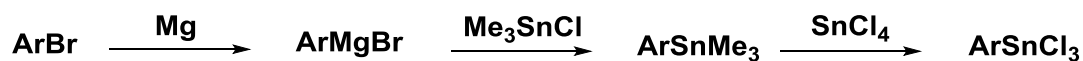
Scheme 36: Synthesis of \text{ArSnCl}_3 on the Grignard route via \text{ArSnMe}_3 as an intermediate.
