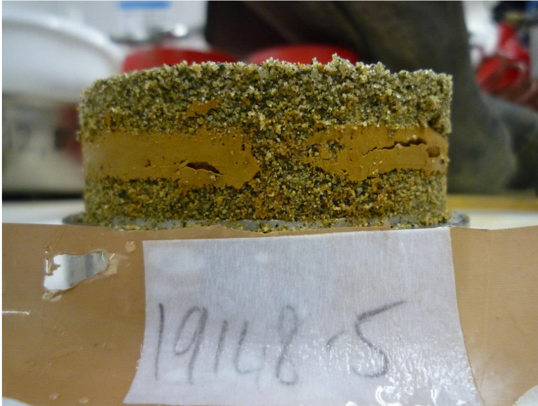
Fig. 26 Post-test state of sample 19148-5; side view.
