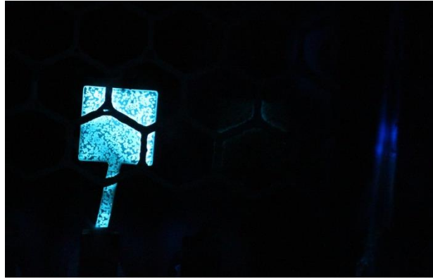
Figure 56: Operating PLED on an embedded copper grid with 2 mm line spacing and 90 \mu\text{m} line width.
