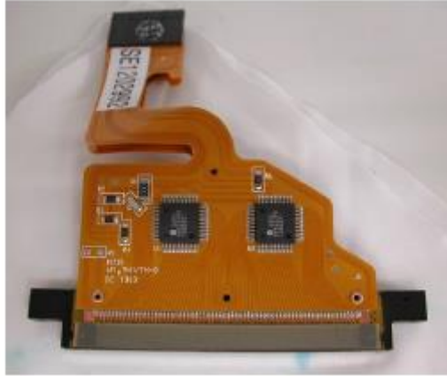
Figure 17: Pix Dro LP50 piezoelectric printhead with 128 nozzles at the NTC Weiz used for this thesis.
