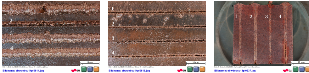
(a) SF-D7; Upper seam; Naht1... Naht4 (top... bottom) (b) SF-D7; Root with noticeable defects (root craters); Naht1... Naht4 (top... bottom) (c) SF-D7; Cross section cut; Naht1... Naht4 (left... right)
