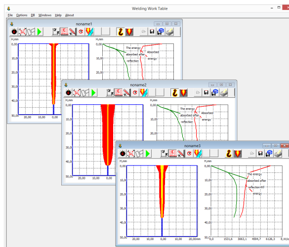
Figure 4.1: Graphical user interface of LaserCAD Version 4.0 with a sample calculation output for an electron beam welding simulation; screenshot from [2]
