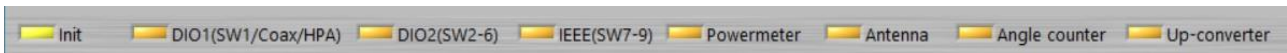
Figure 4-11 LEOSv2 GUI Info area status LEDs in the case of errors during initialization.
