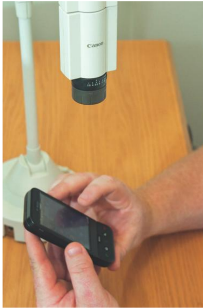
(a) Document Camera for mobile devices usability tests [9].
