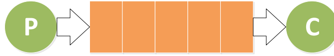
Figure A.2: Block diagram of a simple producer consumer example for AMQP.
