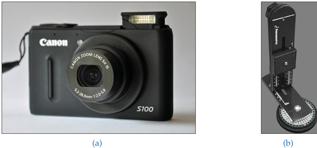
Figure 3.1.: The setup for standard image acquisition, consisting of a Powershot S100 consumer camera (a) and a Panosaurus panoramic head (b). 1
