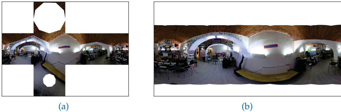
Figure 2.8.: Comparing cubemaps (a) and equirectangular projection (b). Note that the very top and bottom of the sphere were not photographed in this case, causing two holes in (a) and white borders in (b).
