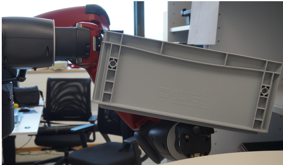
Figure 5.16: This figure shows Baxter carrying a box, where its right arm grasps the box. Its left arm supports the manipulation.
