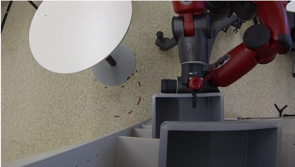
Figure 7.3: This figure shows the top view of the support pose. Within the next step Baxter pulls the box on the support arm.
