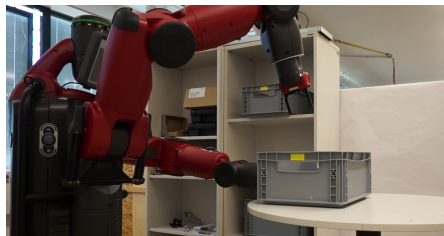
(a) Baxter inspecting the box with its end effector camera.
