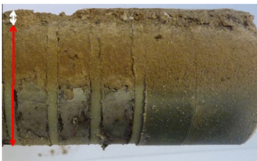
Fig. 4. Photo of the corrosion probe after the forest wood chips test campaign (exposure time 325 h). Explanation: the thickness of the deposit layer is indicated by the white arrow, whereas the red arrow indicates the diameter of the probe; windward side above, leeward side below. (For interpretation of the references to colour in this figure legend, the reader is referred to the web version of this article.)
