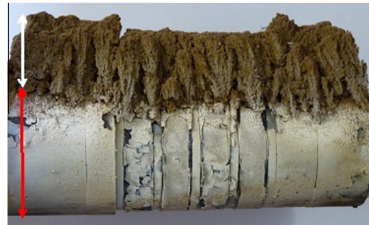
Fig. 5. Photo of the corrosion probe after the waste wood test campaign (exposure time 329 h). Explanation: the thickness of the deposit layer is indicated by the white arrow, whereas the red arrow indicates the diameter of the probe; windward side above, leeward side below. (For interpretation of the references to colour in this figure legend, the reader is referred to the web version of this article.)
