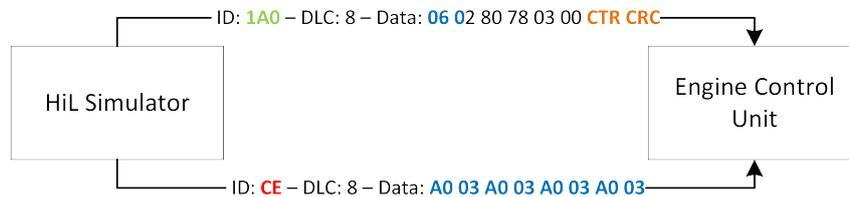
Figure 5.20: Speed related CAN messages with example values used for our attacks in the passenger car HiL system setup. The bold blue numbers within the payload represent the bytes that control the vehicle speed.
