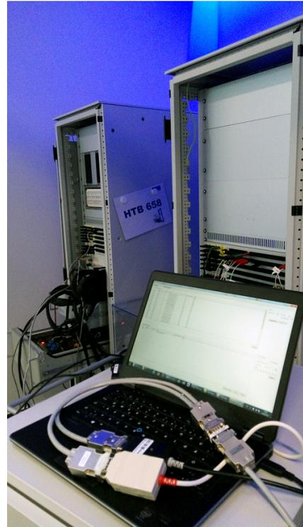
(b) Connecting the CAN-CT via the PCAN-USB adapter
