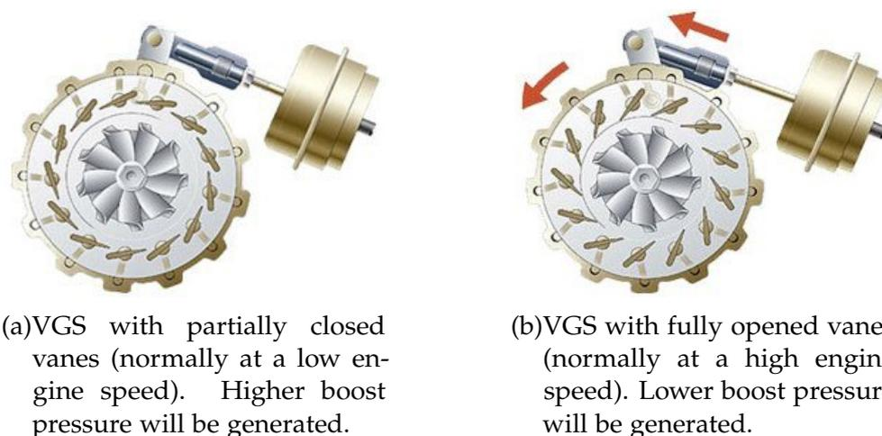
Figure 5.10: Overview of the VGS at high and at low engine speeds<sup>3</sup>
