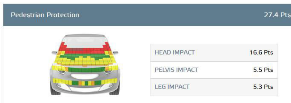
Figure 2-6: Pedestrian protection evaluation Euro NCAP [14]
