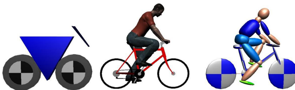
Figure 4-3: PC-Crash abstracted bicycle model, graphical model and multi-body system
