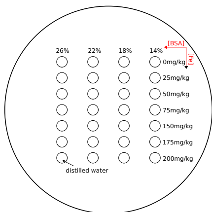
Figure 3.3: Schematic sketch of the cross-section of the BSA phantom. From right to left the BSA concentration increases and from top to bottom the iron concentration increases. The bottom-left cuvette is a sample which contains distilled water as a reference value a bound pool fraction of zero.
