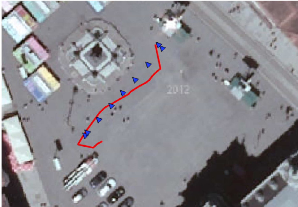
Figure 4.7: Camera poses (blue triangles) after an image based camera pose reconstruction and a global alignment step, based on the method of Horn [28]. The red line represents the sensor based track recording of a smartphones GNSS receiver. Background satellite image from www.basemap.at
