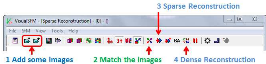
Figure 4.6: Changchang Wu [63] provides here a short instruction of the 3D reconstruction process with his GUI based software VisualSfM.
