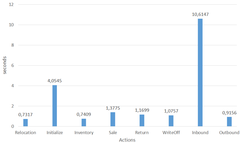
Figure 5.10.: Average execution time for each action in a database with medium size (approximately 5,000 items).
