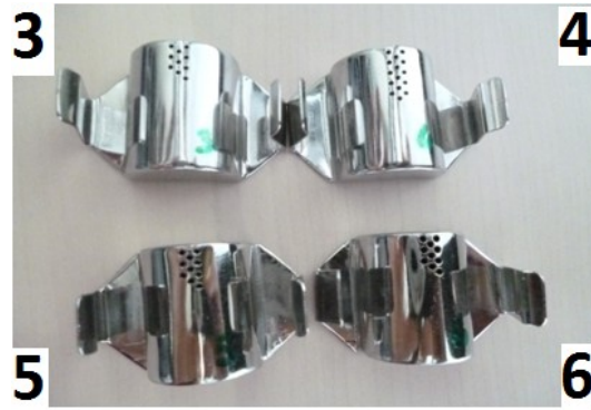
Figure 8:Comparing available sieves for Microdose system. Sieve number 3 with smallest holes' size and sieve number 6 with biggest. Sieve number 4 has the most holes.
