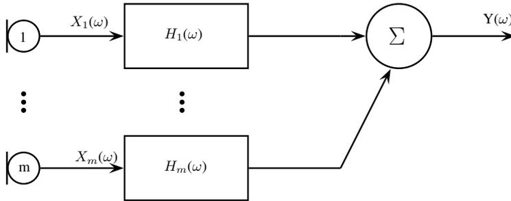
Figure 2.2: Signal model with filters
