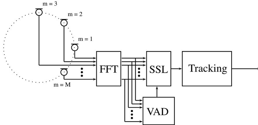
Figure 4.1: Block diagram of a localisation system
