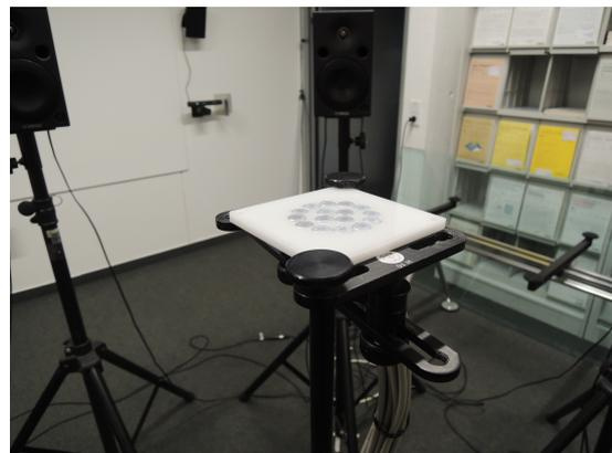
(b) Detail of mounted microphone array
