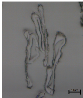
Figure 2.22 Touching softwood kraft pulp fibers digitized using serial sectioning.
