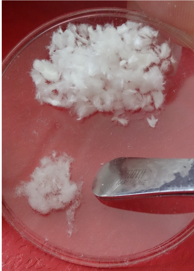
Figure 3.4 Pulp fibers separated from the pulp sheet and pushed together to a fluffy ball prior to embedding.
