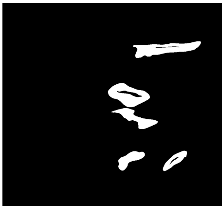
(c) Binarized unbleached softwood kraft pulp fiber cross sections at 10% RH.
