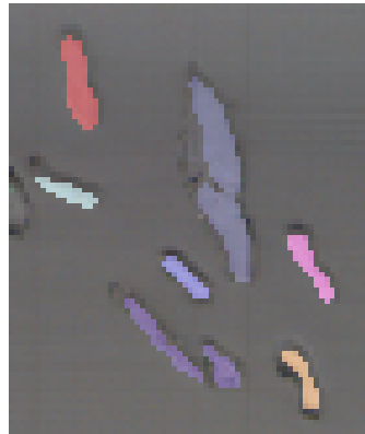
Figure 2.23 Touching eucalyptus pulp fibers digitized using serial sectioning and binarized by the novel segmenter.
