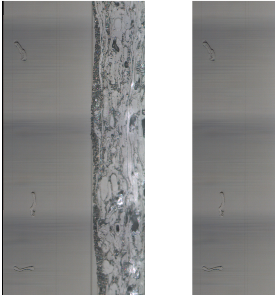
Figure 3.5 Left image: Intersection of digitized sample cross section after stitching and aligning. Three separated fibers are shown on the left side of the sample cross section. The right side of the graphic shows the coated paper's cross section. The coating layer creates a distinctive edge, which is used as a guide bar for the stitching and aligning software. Right image: Image prepared for image analysis. The uneven left side of the image was trimmed, the coated paper cross section on the right side of the image was cut away. Both images have been taken at 50x magnification.
