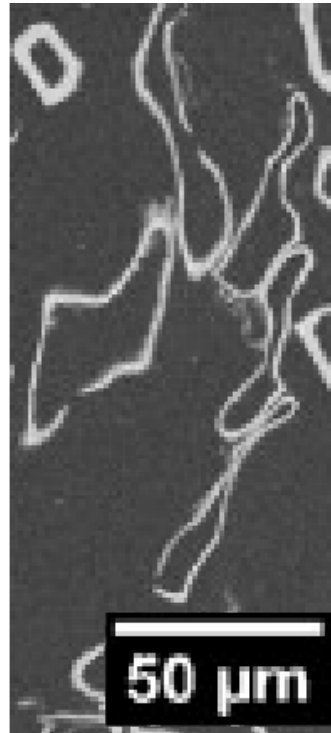
Figure 2.21 Touching mechanical softwood pulp fibers digitized using SEM (Chinga-Carrasco et al. [2009])
