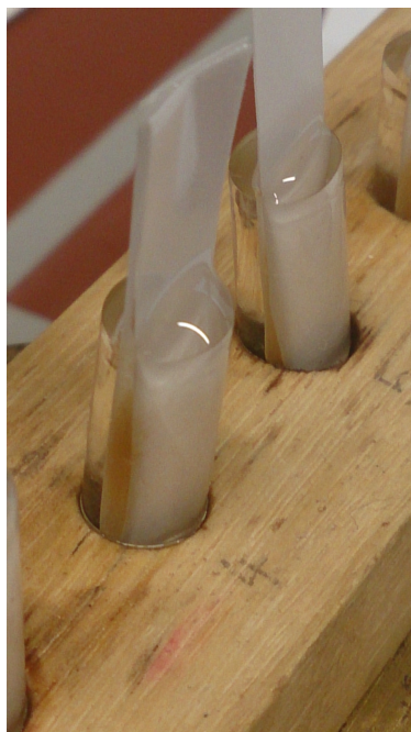
Figure 3.6 Capsules right after grouting with resin, containing the unbleached sample fibers between a folded piece of coated paper that has the function of a guide bar for the stitching and aligning software.
