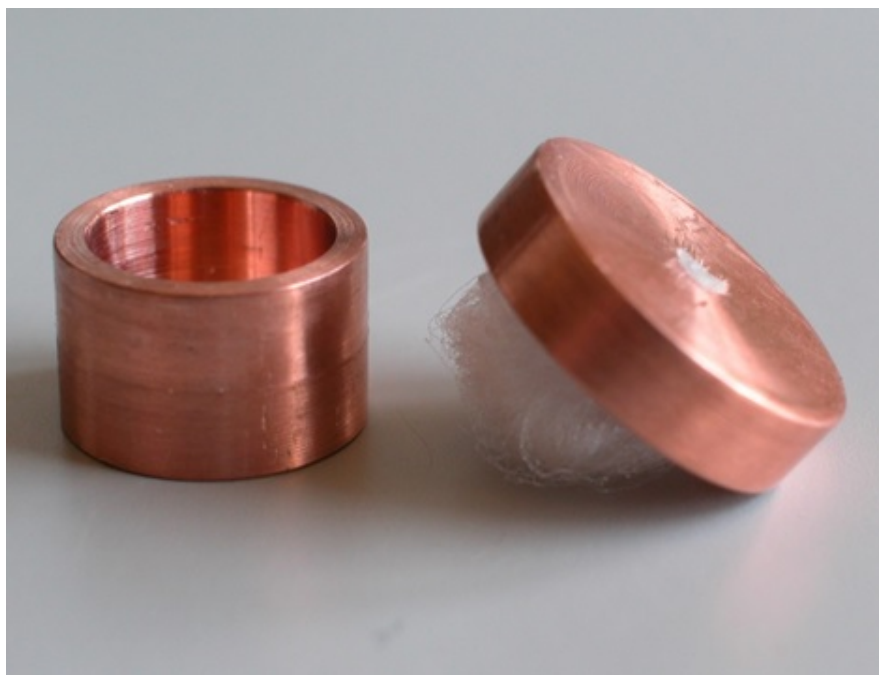
Figure 6.1 Copper lid sample holder with fibers and capsule (Nachtnebel, M., personal communication, April 28th, 2016).
