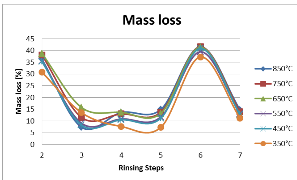
Figure 7 Mass loss during annealing process as a function of rinsing step number (lines are used to guide the eye)
