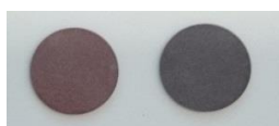
Figure 17 – Visual color change of the material during tempering at 430 °C in air of a PLZT ceramic, containing 0.5 wt.% (2 mol%)CuO
