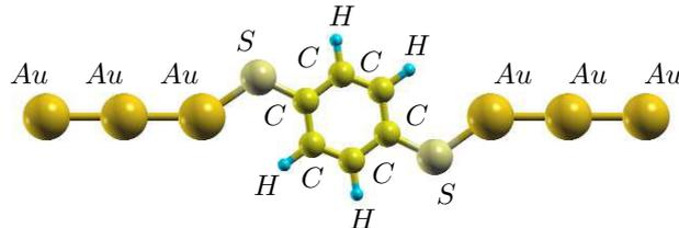
Figure 4.18: Gold-BDT-gold system used for the transport calculation.
