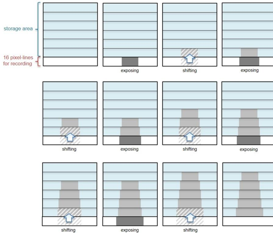
Figure 3.6: Schematic illustration of the image recording procedure to enable fast picture acquisition. 16 pixel-lines of the CCD array are used to record an image, the remaining pixel-lines serve as fast writeable storage to cache the recorded images. After exposing the 16 pixel-lines area the recorded image information is shifted to the storage area. The 16 pixel-lines are cleared and can be reused for exposure.
