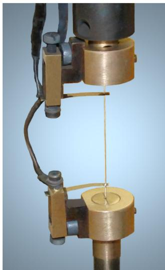
Figure 3.3: Picture of the wire specimen positioned vertically aligned in the sample holder. Two metal foil contacts (knife edge probes) are connected horizontal to the wire surface for voltage drop measurements.
