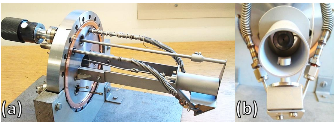
Figure 4.6: (a) Side and (b) frontal view of the semiconductor deposition system. In (a) the rotary double shutter system and in (b) the central Knudsen cell and shielding shroud for simultaneous evaporation onto the quartz microbalance (bottom) and the sample are shown.
