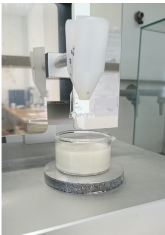
Figure 4.6: Depositing silver nanowires on the cellulose fibers by dip-coating
