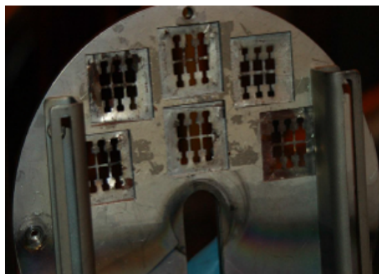
Figure 3.6: Shadowmask used for aluminum evaporation [16]
