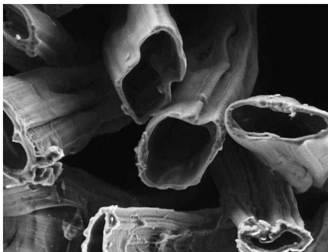
Figure 2.9: Electron microscopy image of the regenerated cellulose fibers used in this study. The fiber diameter is approximately 20 \mu\text{m} . Picture courtesy of Kelheim Fibres GmbH.
